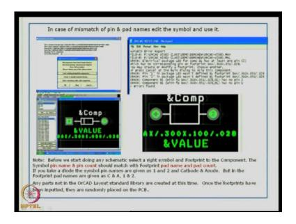
So, in case there is a mismatch between pin and pad names, you edit the symbol and use it. Before we start doing any schematic, select the right symbol and footprint to the component; the symbol pin name and pin count should match with the footprint pad name and pad count; so, this, I have explained earlier. Any parts that are not available right now, needs to be reverted back and then looked at in the schematic.
