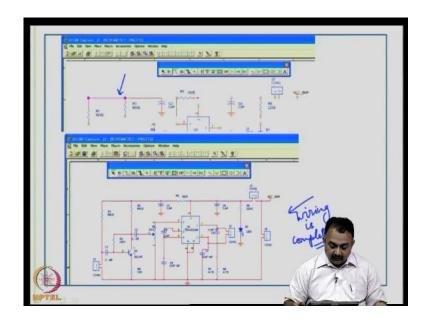
Now, you can start using the command called place wire, which is, you are going to begin to interconnect here; so, this is symbols, done; now you have to start placing the wire; so, go to the place wire tool in your schematic capture and start placing the wires, as you can see here; different components are being connected, according to the circuit diagram, and here you can see, the wiring is complete.
