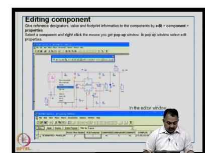
Editing component - when do you require this? The reference designators, value and footprint information to the components can be given by invoking the edit manager or the edit library tool in your particular software, going to the particular component and looking at the properties.
