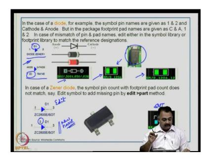
In the case of a diode, for example, the symbol pin names are given as 1 and 2, and cathode and anode, but in the package footprint, pad names are given as C and A; 1 and 2. You must be able to look at these kind of numbering naming systems.
