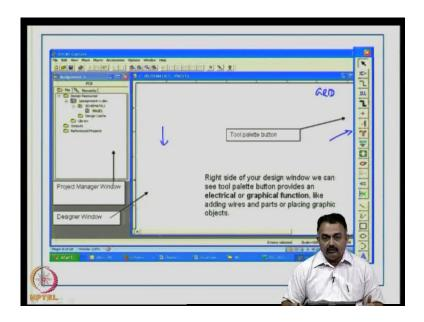
Once you invoke the schematic, you will see a grid here and on the right you will see a palette, which basically contains all the tools; for example, it contains component symbol information, wiring tool, netlist tool, routing tool, a power - ground information insertion, symbols, text editing, various shapes, keep off distances to be drawn, various nonelectrical symbols that you need to create and so on
