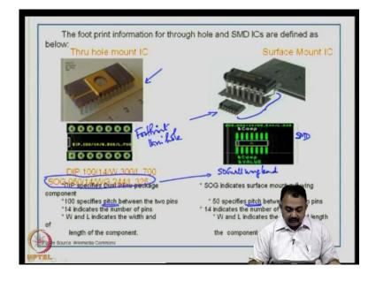
The footprint information for through-hole and surface mount device integrated circuits or active devices are seen here.
