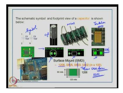
The schematic symbol and footprint view of a capacitor is shown below. This is the symbol, as usual, you are aware of this, for a capacitor. The values are also given 10 microfarad; positive and negative; or it could be 1 and 2.
