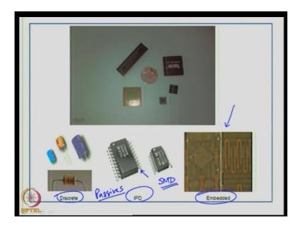
This is again, an example, showing that today, we are moving away from discrete passive devices; these are passive components; we started with discrete devices; we have worked with the integrated passive devices, which means the passive devices are similar looking to a DIP package, but they are integrated inside this housing; and the IO connections are typically in the form of lead frame structures that you see here.
