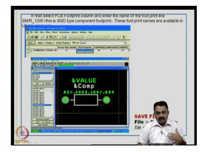
Select the component and look at the properties; and then edit whatever pin information is required, the numbering sequence that is required and so on; and then save it as a new symbol or a part. The same thing can be done with the part library; in the PCB footprint column, enter the name of the footprint; let us say, 1206 SMD resistor; and then you can go there and edit the required information; and save it as a new part.
