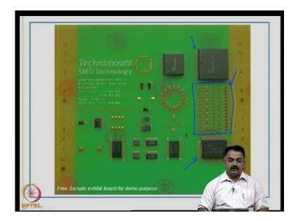
And here, you can see at the middle, there are various capacitors and resistors, very small in size compared to your through-hole capacitors, which are fairly large and they occupy a large area on the board; in contrast, surface mount devices will reduce the board size. That is the exact reason why people are reengineering their through-hole boards to surface mount technology.
