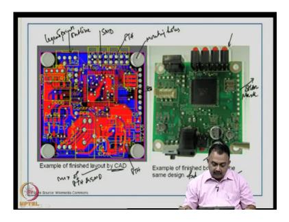
That can help in getting reliable completion. This is a picture that I am giving you as example of a finished layout by CAD whatever things that you can see. On the right, you see the same design has been fabricated and assembled. So, fab plus assembly done here. Here it is a mask. Let us say a CAD view of a layout. You can see these are mounting holes and you can see lot of through hole components.
