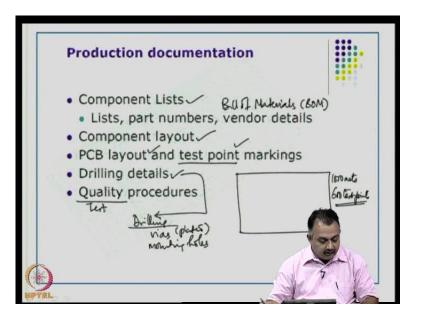
All of these together is an activity called creating technology files. At the end of the routing process, you will create a set of technology files that would be sent to the manufacturer for doing all of these PCB fabrication processes. I hope this is well understood. In any project, whether it is a student project or a industry project or whether it is a research project you have to do a lot of documentation.
