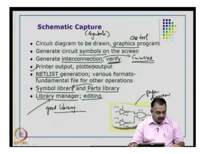
The first thing in a CAD process is that there will be a paper diagram. For example, assume this is the paper diagram that you have of a schematic circuit of an electronic circuit. You have to now do schematic capture using a CAD tool. What you do for that? You have to create a circuit diagram using a basic graphics program that would be available in the CAD tool.
