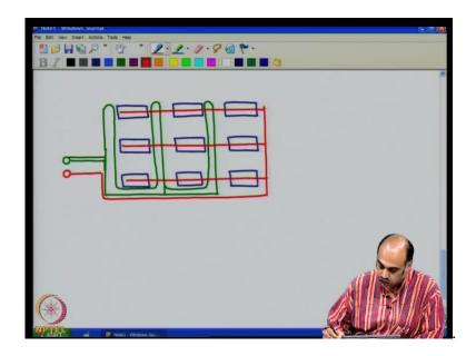
Let us say that we have components laid out in this fashion. It could be integrated circuits ICs or it could be analog components or it could be discrete components - any of them. Let us say we have a matrix of components, which are laid out like this. Let us say one of the lines could be the supply lines. Let us say we have the supply connecter pin here, ground connecter pin here, you could you could go in this fashion. Take the ground you could route the ground like this.
