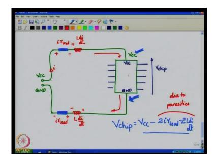
Let us say for example, you have a digital circuit like this. This digital circuit is connected on one side to a  $V_{cc}$  and on the other side to a ground. These  $V_{cc}$  and ground lines are actually tracks which get connected like that. These are also tracks let us say it goes and terminates at a particular connector pin or at some other portion of the Printed
