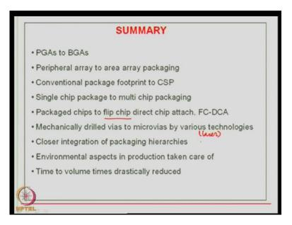
So, summary for this chapter on packages is that, if you have gone through the various sessions that these packages encapsulated. BGA is the work cross, so we are moving from PGAs to BGAs, we are moving from peripheral array packaging to area array packaging. We are moving from conventional package footprint to CSP type of footprint, and CSP pitch as you know is very small, single chip packaging to multichip packaging is the order of the day.
