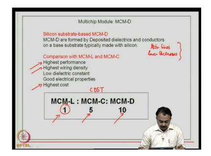
Now, if you look at MCM-D, D stands for Deposited thin film, the fabrication is similar to silicon substrate based process and these are formed by depositing dielectric materials and conductors on a base substrate typically made with silicon. So, it is something like fabricating or using a wafer fabrication process, but on a slightly macro skill because it is a package substrate.
