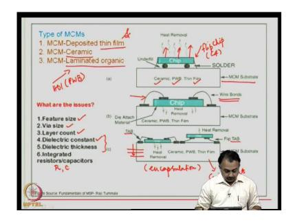
So, here is a picture of a multichip module, where you can see different dies assembled on this surface of substrate - ceramic substrate - and then interconnected, there are also passives that are used in conjunction with the active devices. Now, what are the types of multichip modules; that we can look at, the first thing is known as MCM-D; MCM-D stands for deposited thin film structure, the second one is MCM ceramic which means, that the MCM is built on a ceramic substrate.
