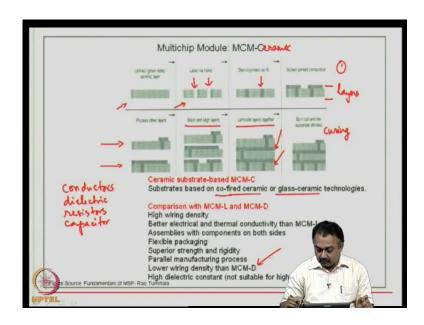
So, the substrate is ceramic, glass composite material, and when we say co-fired what basically happens is, for building MCM-C you require conductors, you require dielectric materials, and then, you may also require resistors and capacitor materials.
