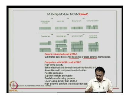
Moisture sensitivity in organic materials is very high, therefore this drawback in terms of electrical poor electrical performance because of moisture absorption is going to be there, but if you look at cost, then people tend to go in for MCM-L. The MCM-C, that is, ceramic process is expensive compared to MCM-L; it is based on co-fired ceramic or glass ceramic technologies.
