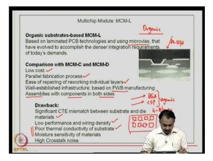
Now, briefly in one slide I would like to mention about the multichip module L type fabrication process. Remember, we are going to discuss these technologies in detail when we look at PWB technologies later. So, in a MCM-L type of structure we are going to use organic substrates, so that is the key part of it.
