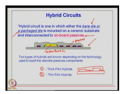
So, this is basically the summary of this particular chapter and before we close I want to introduce a new term called hybrid circuits, which in some sense is closely related to the type of package, that we are - packages that we are aware of - especially, when use ceramic packages, but we will deal with hybrid circuits and MCMs when we come to the technology part.
