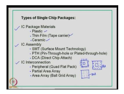
What are the types of single chip packages that are available? They can be classified based on package materials. First thing- it can be a plastic package, the second thing- it can be a thin film or a tape carrier and thirdly- it can be a ceramic material that can be used to package the material, which means in the first case, you are going to use a plastic
