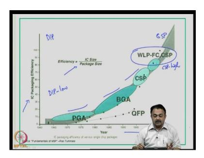
The basic difference between BGA and CSP here is that the package volume is much less in a CSP compared to a BGA. So, today, we are in the era of CSP's. If you look at
