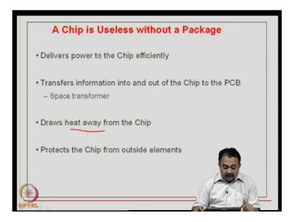
Now, is it really required to use a package? A chip is useless without a package. As many people would like to affirm because it gives you a well defined methodology for system functions like power delivery to the chip efficiently through a much larger pitch and the interconnect device dimensions.
