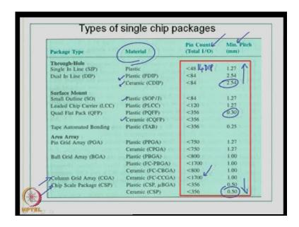
So, the types of single chip packages can now be classified as: through hole packages, which is single in line package, dual in line package and they can be plastic. So, these are the materials that you can think for these package types. So, through hole it can be a plastic package or it can be a ceramic package and then you have surface mount technology, where you have different types and again the types of material that are used is either plastic or ceramic.
