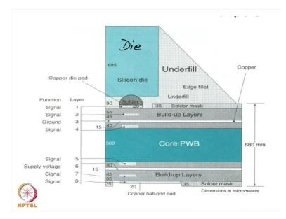
You can see the entire structure is a high density interconnect structure. So, you have an underfill, you have the die, you have the solder mask material, which protects the buildup layers of the PCB. You have the bump here and so on. So, this is a very delicate structure and when you operate or power up this kind of a circuitry, which utilizes a bare die or a package die, obviously heat is generated.
