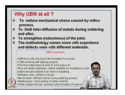
Why UBM at all? It will reduce the mechanical stress caused by reflow process to limit inter-diffusion of materials or metals during the soldering process and after. Then to
