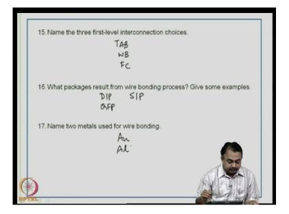
We have seen in today's class about first level interconnections. Wire bond, TAB and flip chip and the second level interconnections are typically taking place at the PCB or the PWB stage. So, the three first level interconnection choices are TAB, wire bond and flip chip. What packages result from wire bonding process? Give some examples, it will be DIP package or a QFP package or a SIP package- Single Inline Package and so on.
