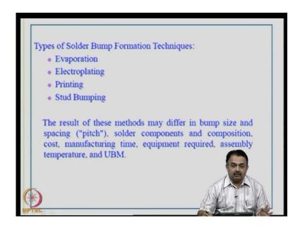
So, the methods to realize the solder bump in these flip chips will be evaporation techniques; typically chemical vapor deposition or evaporation methods. You are familiar that electroplating mechanism and stencil printing mechanism is now available today, where you print these solder paste material and then reflow. During reflow, you can see the bump formation without any solder bridging because of surface tension
