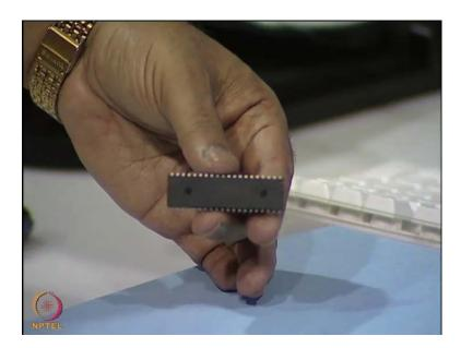
For example, this is an IC you can see here; the very old device this is known as a DIP package (dual in line package) and from here (Refer Slide Time: 25:08) we have moved
