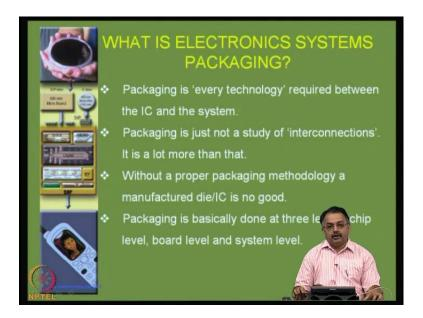
The first bullet says, packaging is every technology required between the IC and the system. Like from a wafer you go to produce integrated circuit - a chip, a device or a microchip or you can call it as an active device which is very essential in any system
