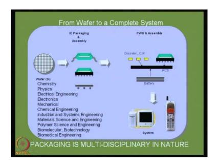
If you look at this slide where I have a depicted how the process goes from a wafer to a complete system. On the left side you see a wafer; I am showing you here a sample of a wafer, a silicon wafer.
