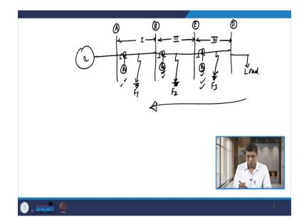
The second type of philosophy that is known as the time discrimination philosophy and here we use time as the coordinating criteria. And the relay we used that is definite time overcurrent relay. The third type of criteria that is the mixture of the first and second that is current time discrimination and in this case we will use both current and time as the coordinating feature. And then we decide the settings of the different relays.
