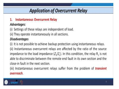
So this is the one of the biggest disadvantage of instantaneous overcurrent relays. Let us discuss the third disadvantage. What is the third disadvantage of instantaneous over current relays so the third disadvantage is this relay all this instantaneous over current relays suffer from the problem of transient over reach. So now, let us discuss what is the transient overreach phenomena.
