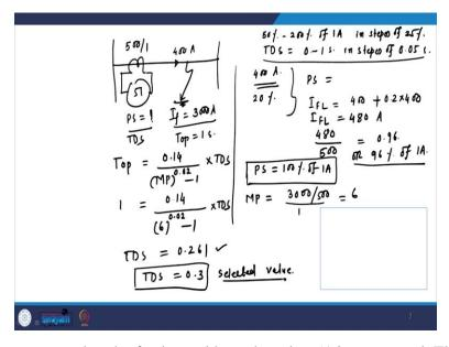
So let us that let us assume that the feeder and here the relay 51 is connected. The CT ratio given that is 500 by one and the fault occurs on this feeder so and the fault current magnitude that is given as 3000 ampere. The relay 51 the setting range is 50 percent to 200 percent of rated current that is one ampere and this is in steps of 25 percent. The time dial setting range of this relay that is 0 to one second in steps of 0.05 second, so this is also given.
