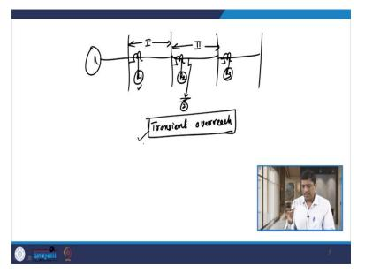
Let us say we have the three line sections and we have the relay same relay R 1 R 2 and R 3 that is connected in three line sections.
