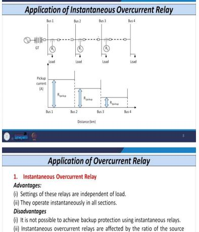
impedance to the load impedance ( $Z_s/Z_L$ ). In this condition, the relay R<sub>1</sub> is not able to discriminate between the remote end fault in its own section and the close-in fault in the next section.
