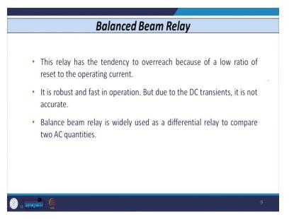
So, this type of relay has a tendency to overreach because it has a low ratio of reset to the operating current. Now, what is the low ratio of reset to the operating current? So, whenever the such type of relay operates, it operates on the principle of Kirchhoff's current law. So, current entering and current leaving to the circuit that remains same.
