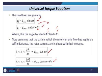
So, if I consider that the flux produced that is phi 1 here in this case this phi 1 that is given by phi 1 max sine omega t, that is one point and the other flux that is phi 2 which is given by the equation phi 2 max sine omega t plus theta. Where theta is the angle between the 2 flux phi 2 and phi 1. So, there are two possibilities either the flux phi 2 leads phi 1 that is one possibility and the other possibility is that phi 2 lacks phi 1. So, that is the other possibility.
