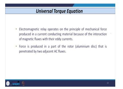
That is known as universal torque equation. So, electromagnetic relay operates on the principle of mechanical force produced because of current flowing in the coil due to interaction of two fluxes with the Eddy currents. So, the force producing one part of the rotor that is the penetrated by two adjacent AC flexes.
