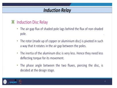
In such a way that it rotates in the air gap between the 2 poles. The inertia of the aluminum disc is very less usually we may use the any type of material for the aluminum disc, but this type of aluminum disc normally is similar to the earlier of electromagnetic type of energy meter. So, they need a very less torque for the movement or operation.
