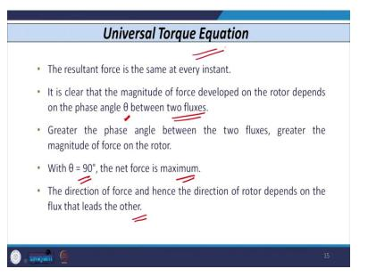
So, this angle theta that plays an important role, greater the this angle between the 2 fluxes, the greater is the magnitude of force because this angle as I told you, it is the sine of angle. So, sine of angle this theta that is maximum when angle is theta is maximum. So, greater the angle between 2 fluxes, greater is the force exerted on the router. When theta is equal to 90 degrees. So, sine 90 that is maximum 1.
