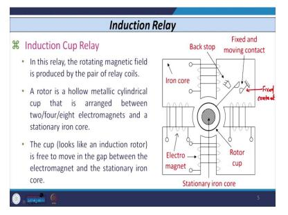
Now, in this relay, the rotating magnetic field is produced by the several relay coils, so we can use so our rotor is a hollow metal cylinder cup that is arranged between either 2 coils either or 4 coils or sometimes 8 coils.
