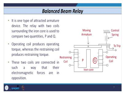
So, as shown in this figure in this balance beam type relay, there are the only 2 limbs of the iron core, the 2 coils are wound as you can see in the figure on the right hand side of the limb there is a one coil which is known as operating coil and it is denoted by the Q. So, Q is known as operating coil and whenever we give this apply to this it is going to produce the flux or force in one direction.
