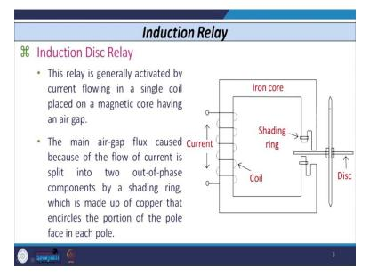
So, if I consider the induction disc relay, then we have the iron core. Now, this iron core is not continuous, but it is basically splitted, so, the air gap is there. And on this iron core the coil is wound and on this coil we are giving the current to the, the core of the this disc relay. Now, if I consider the induction disc type relay, then this relay is generally activated by current flowing in a coil which is wound on a magnetic core.
