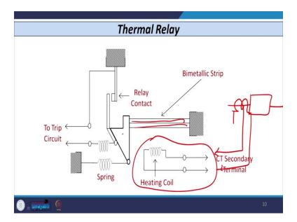
Now, below this bimetallic strip, we have the heating element. So here, this we have the heating element. So this heating coil that is connected to the secondary of the CT. So, if I have the winding of the equipment here and if I have the CT somewhere here inside this, then secondary of the CT that is connected to this heating coil to terminal of the heating coil.
