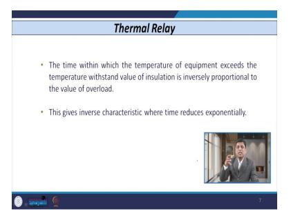
Now, the time within which the temperature of equipment exceeds the withstand temperature or withstand temperature of insulation, that is inversely proportional to the value of overload. So, higher the percentage of overload, lower is the time up to which the, this, the temperature, equilibrium temperature that is reached that takes lower time, that so both are inverted proportional. So if I draw the graph, then we have inverse characteristic of graph between these two.
