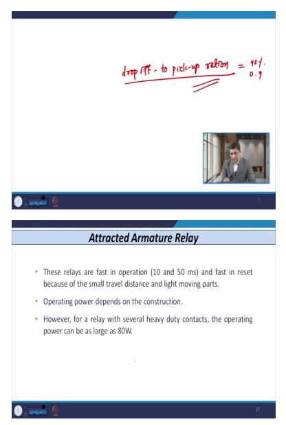
So normally, each and every manufacturer who is manufacturing attracted armature type of relay, they usually provide or they define one term that is known as drop off to pick up ratio. So, drop off to pick up ratio for attracted armature relay that is very high, almost 90 percent or 0.9 in this case.
