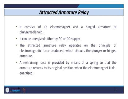
So this type of relay consist of an electromagnet along with some hinged armature or plunger or sometimes it also contains the solenoid. This type of relay is operated by both AC and DC supply. The attracted armature, this type of relay, the working principle is that whenever the current, current-carrying coil that is placed on the core and when it draws a current, it produces the mechanical force and that force is given further or transferred to the relay contacts and hence the relay operates.
