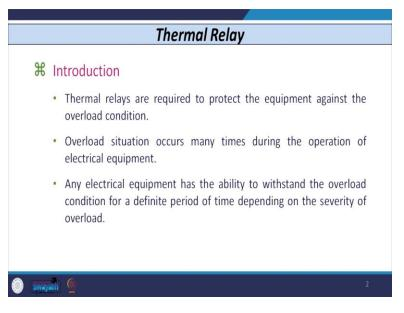
So thermal relays are used basically to protect the equipment against the overload condition. So, now, let us see first what is the difference between overload and fault.
