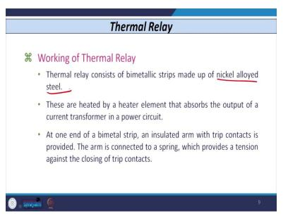
As the name suggest, there are two strip, so it is bimetallic strip, which is made up of the nickel alloyed steel.
