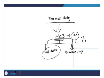
So, if I, if I consider the, if I want to give you just the example of this thermal relay, then we can compare the thermal relay with the function of MCB. So we know that we are utilizing miniature circuit breaker in our, for domestic applications. So, this MCB, if you just look at the circuit of the MCB, then this circuit of the MCB also contains two things. One is the bimetallic strip and the other is the some instantaneous device.
