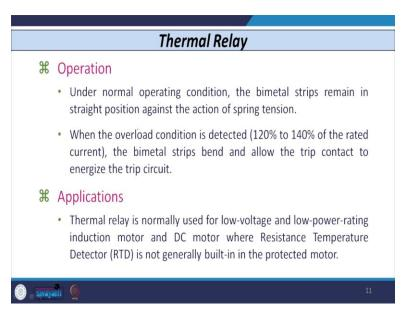
So whenever, under normal condition, the bimetallic strip remain in straight position because this spring will provide some force. Now, whenever there is a overloading of the equipment that means the, whenever the equipment draws the load or current higher than the rated value, say 120 or 140 or 160 percent, then this bimetallic strip bends because they have different coefficient of expansion.
