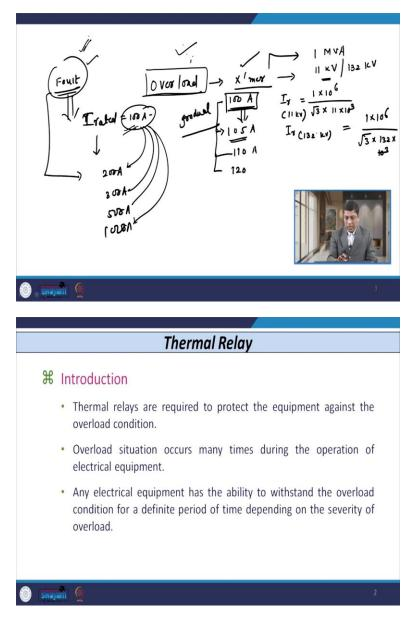
So, whenever I say that what is overload; so overload means if any equipment is there, let us say we have a transformer. Say, this transformer is rated to take the 100-ampere current. Let us say it is, it has some rating, MVA rating; it has some voltage rating, and based on that it is capable to take off the 100-ampere current.
