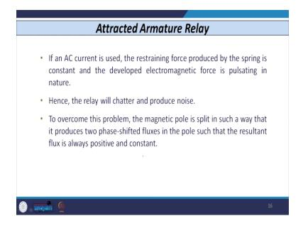
Now, the main important point is that if I use AC quantities for this, means whenever we give AC supply to these coil, then obviously restraining force produced that is produced by spring that is constant, if I assume that is constant, then the whatever force is produced that is pulsating in nature, because we are giving AC supply and every half cycle, the natural current 0 comes by this AC supply.
