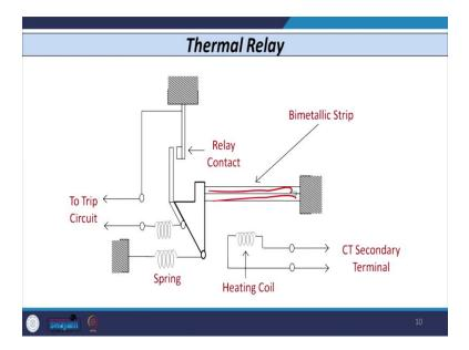
So if I consider just the diagram of thermal relay, then this is the bimetallic strip.
