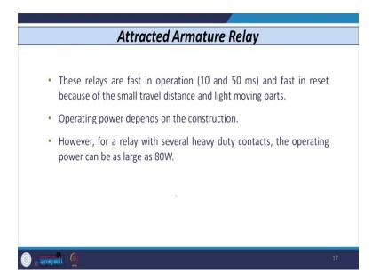
These type of relays, attracted armature type of relays are very fast in operation and the main advantage of this relay is their resetting time, that is very high.
