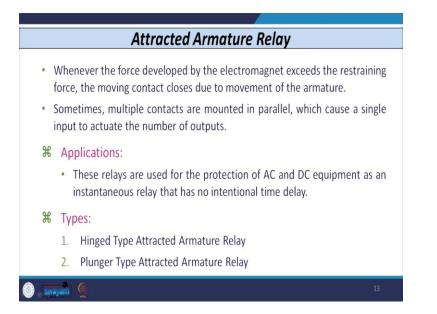
So, whenever the force developed by the electromagnet exceeds some restraining force, this type of restraining force is provided by the spring, then the armature, movement of the armature is there and this movement of the armature that is given to or transfer to the relay contacts and relay operates. So, sometimes multiple contacts, these are also provided and these are connected in parallel to actuate the relay.
