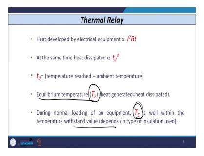
So, that means, whenever this transformer carries or draws a rated current or full load current, the equilibrium temperature TE that is well within the withstand temperature, that is whatever is the insulation provided in the equipment.
