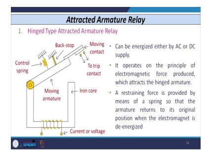
So, hinged type armature relay, as you can see in the figure, there is a coil which is placed on the core, iron core, and from this coil we give either current or the voltage depending upon what type of relay we want. And on one side of this core, the one moving armature is connected, so this moving armature is controlled by spring and backstop and one other side of moving armature, the moving contact of the relay that is connected.
