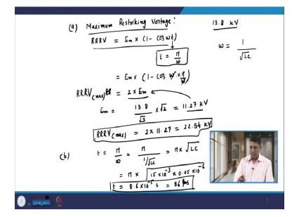
So as I told you earlier, that the, in this equation, the maximum Restriking Voltage occurs at t is equal to pi by omega. So, we have the pi, what is omega? As I told you, omega that is equal to
