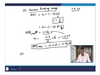
So, the first part you need to find out the maximum Restriking Voltage. So, the maximum Restriking Voltage that is nothing but as I told you, it is your RRRV. So, we have already considered the equation of RRRV. So, the equation of RRRV that is given by the Em, the maximum value of the voltage into 1 minus cos omega t. So this is the equation of RRRV and the value of RRRV that becomes maximum when you have the value t that is t is equal to pi by omega.
