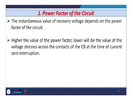
So if I just consider the power factor, then we know that the instantaneous value of Recovery Voltage depends on the power factor of the circuit, higher the value of power factor, lower is the voltage as trace appear or existing on the across the contact of the Circuit Breaker at the time of interruption of current at natural current zero.
