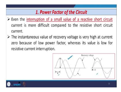
So, the instantaneous value of recovery voltage is a very high at current zero because of low power factor whereas, its value is low for the resistive current interruption. So, you can see that I have shown the two important waveforms. The first waveform you can see that the value of phi that is very high. So, the angle between recovery voltage and the current to be interrupted that is very high. So, power factor is very low because of course phi is very high so, cos phi is very low.
