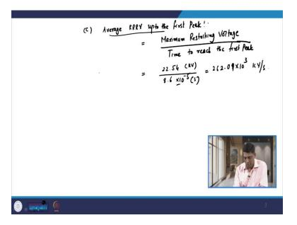
So let us see this third part that is C, that is the average RRRV up to the first peak. So the average RRRV up to the first peak that is given by the maximum Restriking Voltage, which we have already calculated in part A and then divide it by the time to reach the first peak. So, the maximum Restriking Voltage we have already calculated that is the 22.54.
