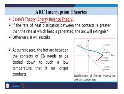
So now let us consider the second type of theory that is given by Cassie's. So, this theory is also known as the Energy Balance Theory. So, in this case, if the rate at which the heat dissipation across the contact of circuit breaker that occurs if that is greater than the rate at which the heat generated, then the arc that is going to be extinguished, otherwise the arc restrikes.
