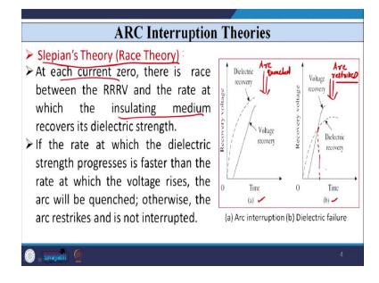
If I just consider this Slepian's Theory, it is also known as the Race Theory. Why it is known as Race Theory? Because whenever the arc is formed across the contact of Circuit Breaker, then there is always a race between the Rate of Rise of Restriking Voltage that is the voltage appears across the contact of Circuit Breaker and the dielectrics or recovery of the dielectric medium that is used in that Circuit Breaker to quench the arc. So there is always a race between this two.
