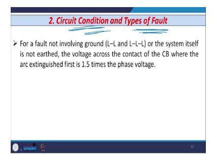
So, let us now consider the second factor that is going to affect the RRRV, Recovery Voltage and Transient Restriking Voltage. So, the second point that is the circuit condition and the type of fault So, okay this is also very important point that is the type of fault and what is the circuit condition means, what is the condition of the parameters whether the system is earth or system is not earth that type.
