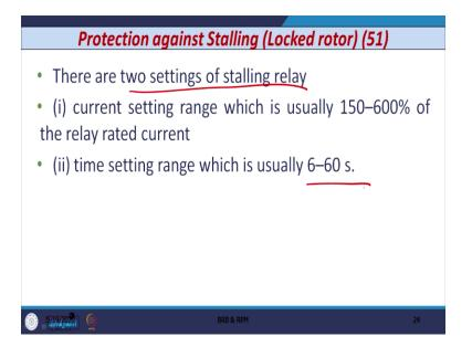
Two settings are provided in the stalling relay, the first that is the current setting, basically it is related to I stall and its range that is usually 150% to 600% of the relay rated current and the time setting range which is usually provided in 6 to 60 seconds in steps of 5 or 10 seconds.
