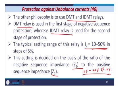
So, the other philosophy, suppose if I have small motors and its cost is low compared to the other motors, then it is not economically viable to use the negative phase sequence relay for protection against unbalanced currents. So, in that case, we may use the definite minimum time delay relay or sometimes inverse definite minimum time delay relays.
