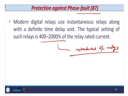
So, protection against phase fault in modern digital relays that is normally dealt with the differential relay and typical setting that is 400% to 2000% of the rated current. So, this setting is normally for the instantaneous relays, instantaneous over-current relays.
