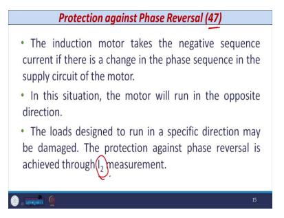
Now, the next type of protection or phenomenon that is known as protection against phase reversal. So instead of giving RYB phase sequence, you -- if the phase sequence is altered or changed, then motor needs to be protected. So for that the relay number given to the protective device that is 47, so the induction motor takes negative sequence current if there is a change in the phase sequence in the supply circuit of the motor.
