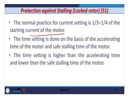
The normal practice for current settings that is I stall setting that is one-third to onefourth of the starting current of the induction motor. So the time setting on the other hand that is done on the basis of the accelerating time of the motor and safe stallings time of the motor. So time setting should be such that should be higher than the acceleration time of the motor and it should be lower than the safe stalling time of the induction motor.
