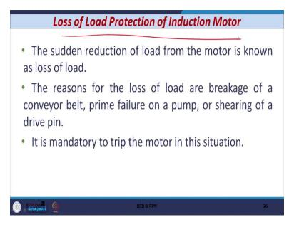
The next point or phenomenon that is known as loss of load protection of induction motor. So the sudden reduction of load from the motor that is known as the loss of load, maybe loss of load that is because of the breakage of conveyor belt or maybe because of the prime failure of the pump or shearing of the drive pin. So it is mandatory to trip the motor in this situation. When load that is suddenly taken away from the motor.
