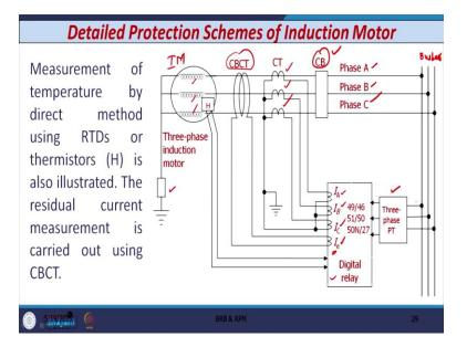
So, if I just draw the detail protection scheme of induction motor, then you can see here is the scheme, so this is the busbar and along with this busbar you have the three phase that is A, B and C, three phases are there along with the circuit breaker. And you have the induction motor here, this is your induction motor that is grounded through some resistor or reactor. These are the three windings of the induction motor.
