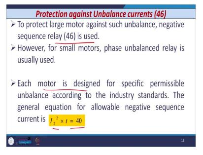
So, to protect the motor against such type of unbalance, negative sequence relay 46 that is used. However, for small motors, phase unbalanced relay that is usually used because it is not economically viable to use negative phase sequence relay for small motors. So, in negative phase sequence relay each motor is designed for specific permissible unbalanced current according to the standards.
