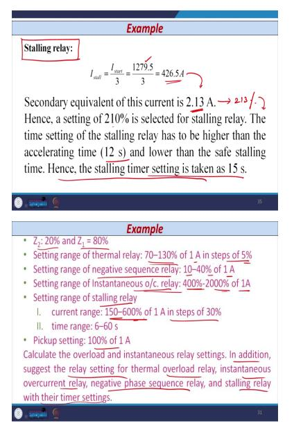
Now, let us consider the setting of the stalling relay or stalling protection. So, as it is specified that the stalling current that is the one-third of the starting current of induction motor. So we have already calculated starting current of induction motor. So, you take one-third, the value comes out to be 426.5 ampere. If you transfer this value on CT secondary side by dividing with 200, then the value comes out to be 2.13 ampere.
