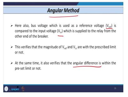
In the second method that is the synchro check method, the angular method is used. So, here the again the same thing is that the bus voltage is used as a reference that is V ref and the line voltage that is used as a V input voltage, and you need to compare these two. So, this verifies the magnitude of V reference and V in. And if this is within the prescribed limit or not that need to be checked.
