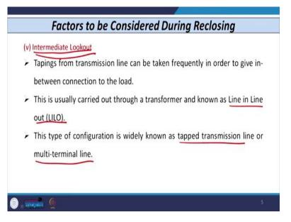
Now, the fifth factor which is very important that is known as intermediate lockouts. Now, what is intermediate lockout? Now, we know that the tappings from transmission line or maybe distribution line also that can be taken very frequently and this is required because we need to provide the connection to the load in between.
