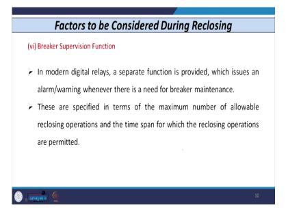
So, once a relay has this number, then it can automatically issue the alarm or warning that okay now there is a need of the breaker maintenance and the operator has to take care of such warning or alarm. So, this are specified in terms of maximum number of allowable reclosing operations, and the time spam for which the reclosing operations are permitted.
