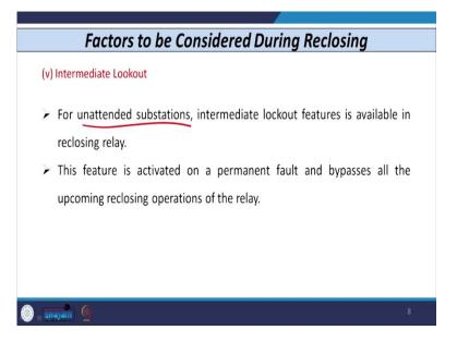
So, on the other hand if I consider the unattended substations and where we have such type of transmission or distribution configuration exist like tapped or multi-terminal lines then intermediate lockout feature that is easily available in the reclosing relay, so this feature is activated in case of permanent fault only.
