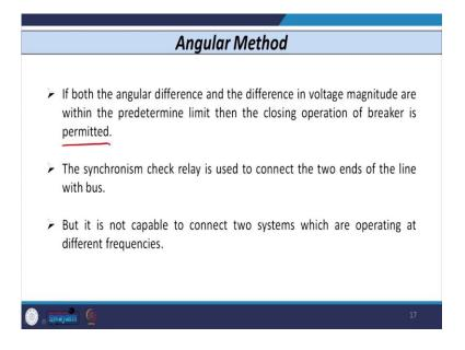
If both the angular difference and the difference in the voltage magnitude are within the predetermined limit, then the closing operation of the breaker that is permitted. If the difference is beyond the limit then the cruising operation that is not allowed. And sometimes nowadays, along with this synchro check relay or element, the interlocking is provided, so that will be done automatically in the unattended substation.
