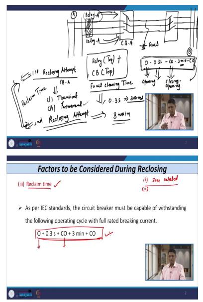
So, let us assume that we have three phase circuit and we have the breakers that is here at this end, and then we have the line and again we have the breakers at this end, and then we have this is connected with the bus. So, we have the three lines. Now, this is the your breaker equipped with auto reclosing facility and this is also the breaker equipped with auto reclosing facility. This is your substation A and this is your substation B. Now, what is the meaning of this sequence.
