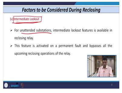
So, that means, what will happen if suppose we have a breaker here, breaker here and we do have a breaker here also if we have a source over here. Now, wherever permanent fault occurs on any of this subsection of this tapped line or multi-terminal line, this breaker that remain in open condition that breaker becomes open.
