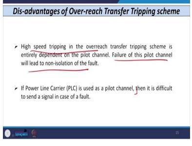
Overreach transfer tripping scheme is advantages compared to under reach transfer tripping scheme because using this you can achieve the high speed tripping of on both the side of the relays. The only disadvantage of this scheme is that if your communication channel fails, then there is a probability of mal operation in case of the default on beyond the zone of the each side of the line section that is F2 or F3. Otherwise there is no disadvantage of the overreach transfer tripping scheme.
