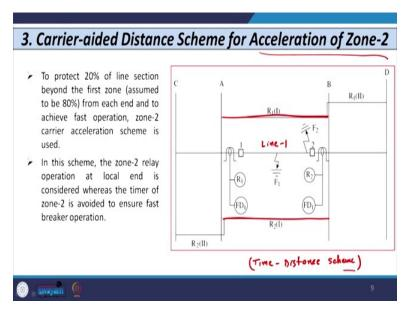
So, this is the time distance characteristic of the carrier-aided distance scheme for acceleration of zonetwo right, this is time distance scheme or characteristic. Now, you can see that I have shown here the same similar diagram time distance diagram the only difference is the first zone, I have extended almost up to the 95% or 100% of the line to be protected, so this is the line which we need to protect.
