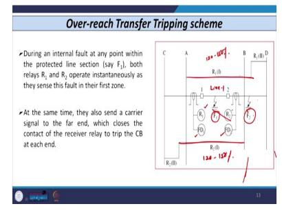
Now in case of external fault at F2 say here, somewhere beyond the zone between any adjoining line section, say line section two.So in this case if fault occurs at F2, then the relay R1 operates in its first zone because that will detect this fault in its first zone because you can see the reach of R1 that is 120%. So R1 that is going to detect this fault in its first zone.
