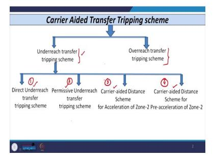
So carrier transport tripping scheme that is classified as one is known as the underreach transfer tripping scheme and the other is known as overreach transfer tripping scheme.
