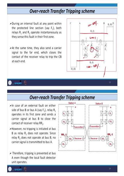
So, with this background, let us discuss the last scheme that is known as overreach transfer tripping scheme. So, as I told you in case of overreach, the first zone reach of relay R1, that will go beyond the line section, so here this is the line to be protected. Similar the first job of relay R2 that will go beyond the line section, the usual setting is 120% to 150% each side.
