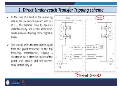
So, what will happen that if fault occurs at F1, this is the control circuit of the direct underreach transfer tripping scheme. So, if fault occurs at F1, which is the first zone of both the relays R1 and R2, then what will happen relay R1 operates so these two contacts that closes here, similarly, fault detector one at bus 1 also operates because current exceeds the predetermined limit, so these two contacts also closes.
