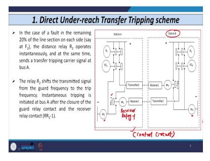
So, if fault occurs on either side of the 20%, let us say, the fault occurs at F2 somewhere here then in this case, as the fault is at F2, so, relay R2 detects that fault in its first zone and it operates instantaneously. So, as R2 operates the fault detector unit at bus B that also operates so this closes and direct tripping command is initiated and the coil of 86(2) that is energized.
