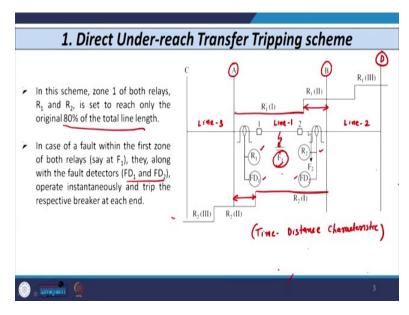
Now, in case of remaining 20% of the line section that means if fault occurs in this section or fault occurs in this section then let us see, how we can achieve the instantaneous tripping, which is not possible if we use the conventional distance relay scheme.
