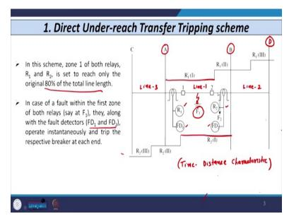
Now, if I consider the underreach transfer tripping scheme, let us discuss the first scheme that is the direct underreach transfer ripping scheme. So, let us discuss the first one, that is the underreach transfer trip scheme. This is the time distance characteristic of the underreach direct underreach transfer tripping scheme.
