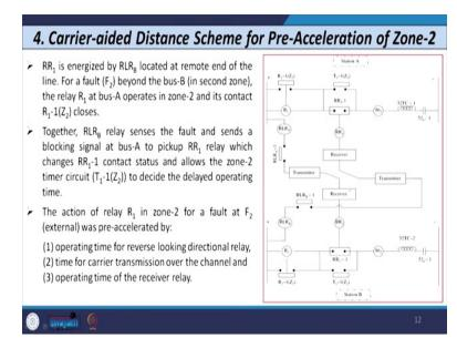
So, if I just look at the control circuit of this, then the RR1 that is energized. So, you can see that the RR1 coil that is available here, so this coil of the receiver relay one that is energized, which is located based on the signal received from the remote end that is from substation B, right, and so really R1 at bus A operates in zone two and it is contact R1-1, Z1 that closes. So R1-1, Z1 that closes so the contact of this relay R1 this contact that closes.
