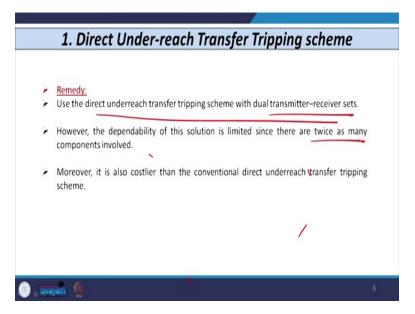
So, what is the remedy? So remedy, one of the easiest remedy is we use the dual transmitter and receiver set under the direct underreach transfer trip scheme, but again, as we use dual transmit set of receiver and transmitter so the cost of this scheme increases compared to the conventional direct underreach transfer tripping scheme, so, and hence this type of scheme that is not used.
