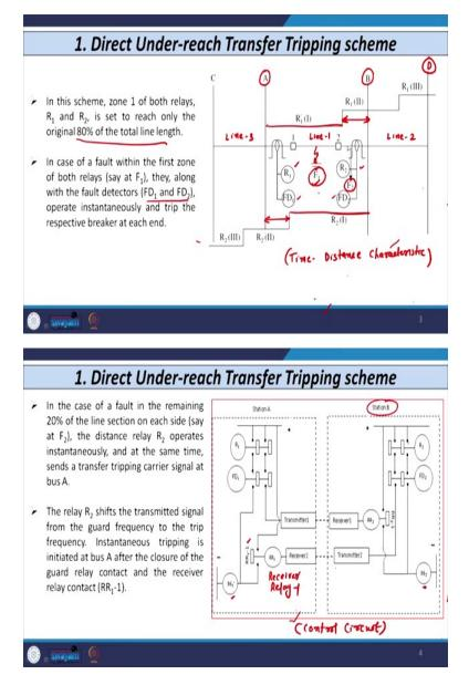
So, you can see that if fault occurs in remaining this 20% that is we have seen at F2 then the relay R2 energize, which R2 senses the fault and that will give signal to the breaker situated at substation B at the same time it also gives the transfer tripping signal at other substation at
