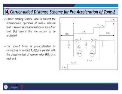
Now, let us see the fourth scheme which is known as the carrier-aided distance scheme for pre-acceleration of zone two. Now, what is the difference? Now in case of carrier blocking scheme, we know that we have already discussed the carrier blocking scheme that is used to prevent the instantaneous operation of zone two means any fault occurs on F2 remaining 20% on this side or this side.
