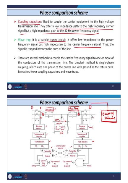
So, the main function of the wave trap it is a basically a parallel circuit and it provides low impedance for the fundamental frequency component and high impedance to the high frequency carrier signals. So, whatever your fundamental frequency component signal is there, all that signals that is available or given to the relay or available with the relay or CT.
