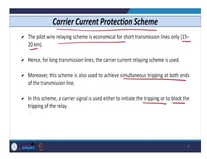
So, instead of that, nowadays, utilities that is using the scheme known as the carrier current based protection scheme. So, let us discuss now, what is the carrier current based protection scheme. So, as I told you, this type of scheme is used in place of the wire pilot relaying scheme, because we can use only up to 50 to 20 kilometer. If I use carrier current based scheme, then again, we can have the simultaneous opening of breakers at both the ends, that is also possible.
