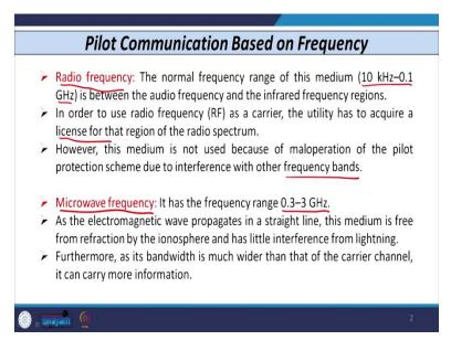
We have discussed based on we can transmit depending upon what type of signal we use either analog digital or we can also transmit based on what is the frequency we can use. So, let us continue with our radiofrequency that is the frequency based pilot. So, when we use the Radiofrequency, the normal frequency range of this radio frequency if I use radio frequency signal for carrier, then its range is from 10 kilohertz to 0.1 gigahertz.
