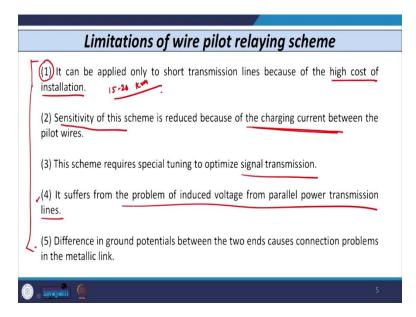
So, the major disadvantages of this wire pilot relaying scheme. The very first disadvantage that is, it can be applied only for short transmission line. We cannot use for long transmission line, because we have to physically lay down the wires. So, its cost is very high, that is why it is used only up to let us say 15 to 20 kilometer short lines or particularly cables.
