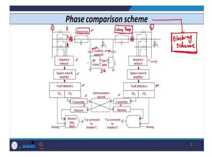
Now, let us see one specific type of phase comparison scheme. And here this type of scheme, we have used this scheme as a blocking scheme. So, face comparison scheme here you can use as a tripping scheme also. But here whatever diagram I have shown, that is a phase comparison type of scheme. And we have used the carrier signal to block the operation of the relay, that is why I told you it is a blocking type of scheme.
