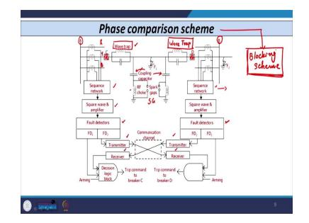
So, as I told you, the spark gap that is used for the protection against over voltage. Now, we do have some other device also. You can see here, we have a square wave and amplifier. And we have some sequence networks also. This sequence network, as I told you while in wire pilot relaying scheme, this is nothing but your summing transformer. So, basically it converts three phase circuit into single phase circuit.
