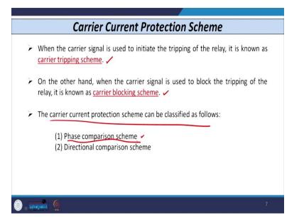
So, when the as I told you, when the carrier signal is used to initiate or start the tripping of the relay, then that is known as carrier tripping scheme or sometimes carrier intertripping scheme. And on the other hand, if I use the carrier signal to block the operation of relay, then that type of scheme that is known as the carrier blocking scheme.
