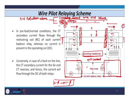
Now, with this discussion, let us start our first discussion scheme, that is based on pilot protection scheme. So, as I told you, the pilot protection scheme that is classified in three types. One is known as the circulating current wire pilot relaying scheme. The second one is the opposed voltage wire pilot relaying scheme and the third is the Translay type of scheme. So, out of this, let us discuss the first one only, that is circulating current wire pilot relaying scheme.
