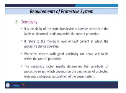
So, sensitivity is nothing but the ability of protective device to operate correctly for any fault or abnormal condition inside the zone of protection. So basically, it is related to the minimum level of fault current at which your protective device operates. So, protective device with good sensitivity can sense any faults within the zone of protection.
