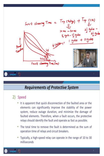
So, if I consider the fault clearing time, then fault clearing time, fault clearing time, that is nothing but the summation of time of operation of protective relays plus time of operation of circuit breakers. So, usually, if I consider the relays, then time of operation of protective relays varies from 10 millisecond to 30 millisecond. So if I consider 50-hertz system, then in that case, the time of operation of relays that varies from half-cycle to the one and half cycles.
