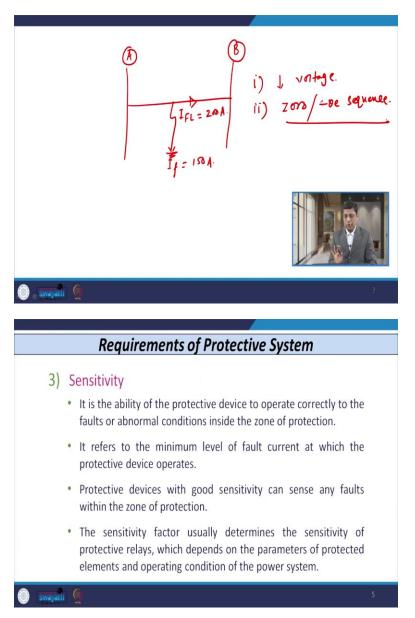
So, for example, if I consider, let us consider the one transmission line connected between bus A and bus B. Say, let us also assume that the full load current of this line that is, 200 ampere. That means this line can take 200 ampere continuously without any damage, without any temperature rise. Now, if fault occurs on this line and let us say, the magnitude of fault current that is, 150 ampere.
