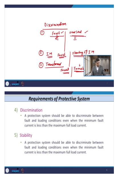
So, to understand this, let us consider, when I say discrimination, then in this case, discrimination can be between either fault and the other phenomena like overload. So, fault means, we know that fault is defined as, it is the abnormal stoppage of current or undesired flow of current that is known as fault. Whereas, in case of overload means gradual increase in load above the rated value. So, there is a fundamental difference between fault and overload.
