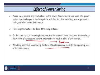
So, now, let us see the another effect, what is power swing. So, power swing causes the large fluctuation in the power flow, that is between two areas. And this fluctuation is maybe because of the change in magnitude of load or direction, switching off line, very big line, loss of generator maybe because of fault or maybe because of some other the system disturbance.
