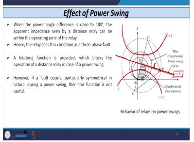
Now, to understand the power swing phenomenon, you can look in this figure. I have shown the 3 zone characteristic of MOH relay. So, this is first zone, second zone and third zone of MOH relay. And I have also shown with dotted line, the quadrilateral characteristic. And I have shown the Locus of Power swing, that is shown by the value R, this R is nothing but the ratio of sending an voltage to the receiving end voltage magnitude.
