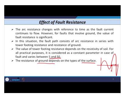
So, the arc resistance changes with reference to time as the fault current continues to flow. So, whenever, if I consider, say fault occurs from this instant. This is the instant when fault occur so magnitude of current that becomes very high. So, from this incident, if you just take one cycle or one and a half cycle, then the value of arc resistance is very small.
