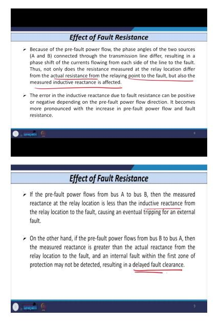
So, this is very important that when we consider the pre-fault power flow, the phase angle of because as I told you phase angle of the two sources connected at bus A and bus B are different. So, that is why both the current IB and IA are not in phase. So, that means because of that, what will happen, not only the real part of the measured value, but the imaginary part of the measured impedance that is also affected because of the impact of fault resistance. So, that means, we can
