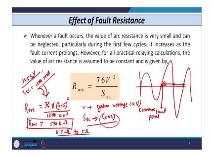
Now, wherever fault occurs, the value of arc resistance is very small. And so, generally we neglect it, particularly during first few cycles, after the inception of fault, we can neglect it and it increases as the fault current prolongs. So, if I consider again, this point which is the fault occurs at this instant. So, this is the occurrence of fault point.
