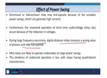
So, whenever power swing phenomena occurs, the current increases. So, any overcurrent relay that is not able to operate correctly. In this case, in case of power swing, voltage also reduces. So, any voltage-based relay that is also not operate correctly. In case of frequency accessors, digital distance relay that also measures the wrong value, because it is based on the phasor calculation.
