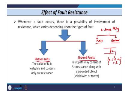
So, as I told you earlier, whenever fault occurs, the possibility of involvement of resistance varies depending upon the type of fault. So, as I told you, the distance relay, if I consider the distance relay, then the distance relay that is of two types, one is phase type distance relay, that means, distance relay as phase unit and another is it has the ground unit. This, we have already discussed.
