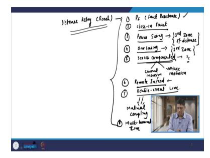
So, if I consider what are the different impacts of distance relay, then the performance of distance relay, we can say the reach of distance relay, that is affected by many parameters. The first that is known as the fault resistance RF. So, that is fault resistance, because whenever we consider the performance of the distance relay, we consider the solid fault. But whenever fault involves some resistance, then it's a reach that is affected.
