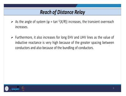
The, it is also true that as the angle phi which is 10 inverse X by R increases, the transient overreach also increases. And for our long UHV and EHV line the inductive reactance is very high, so obviously the spacing between the conductors increases, due to, because of utilization of bundled conductors, so the value of transient overreach also increases. Now, with this background let us see, what are the different types of distance relay characteristic that is available in market.
