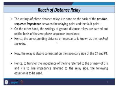
We know that the relay is always connected as I told you on the secondary side of CT and PT or CBT. So, we need to transfer the impedance from primary side to the secondary side because the impedance seen by relay that is different and impedance on the, of the line which is on primary side that is also different. So, if I want to just convert the, this impedance from primary to secondary side, then we need to use the equation.
