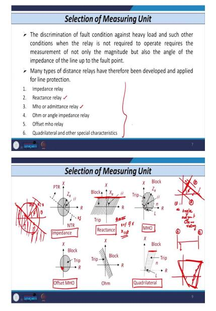
So, let us discuss different types of characteristic. So, usually there are six characteristic, it can be more also, but let us restrict up to six only. So, the first characteristic is known as impedance type distance relay. So, if I use the impedance type distance relay, then this characteristic is shown here, this is the impedance type distance relay characteristic and you can see that there is a circle on the RX plane.
