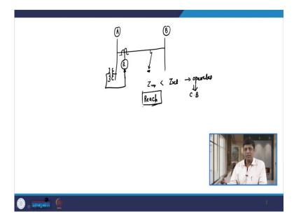
So, whenever any distance relay we put in the circuit then in that case, if I consider, let us say a bus A which is there is a line connected between A and B and we put one distance relay here R, which is also fed by the line PT also. Obviously, whenever fault occurs on the line, the distance relay, just measure the impedance and when the measured impedance is less than some set value of impedance, then relay operates.
