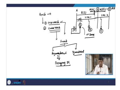
So, we have discussed, what is the reach of the relay. So reach means the area or portion up to which relay is able to sense the fault. Based on this we have another two important definition one is known as overreach, and the other that is known as under reach. So, what do we mean by overreach? So, again let us consider the same example where we have connected a line between A and B, we have another bus C, so we have another line say this is line 1 and this is line 2.
