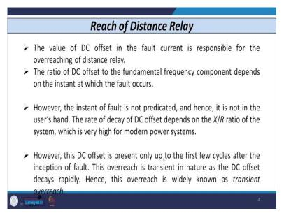
So, this decaying DC component is responsible for the whether relay overreaches or relay operates correctly. So, the value of this decaying DC or DC offset in the fault current that is responsible for this overreaching of the relay. The ratio of DC offset to the fundamental frequency component that depends on the instant at which fault occurs. So, if I (just), if we
