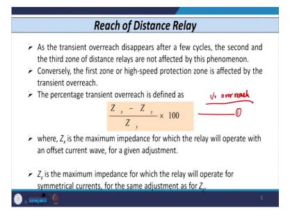
So, how to find out this percentage transient overreach? So that can be obtained using this equation. So, in this equation, you can easily find out the value of percentage overreach that is for any distance relay. So, in this case Z x that is the maximum impedance for which the relay operates with an offset current wave for an (adjacent), for a given adjustment and Z y is the maximum impedance for which the relay operates for symmetrical current for the given
