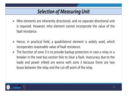
So, as I told you Mho relay is inherently directional and it can also accommodate some marginal value of fault resistance also, so it is used for longer EHV and UHV transmission lines. However, nowadays we know that we are utilizing digital relay and all earlier electromechanical and static type of relays are replaced by digital relays. So, whenever we use digital distance relay in actual field then this relay has different types of characteristic like quadrilateral, elliptical, quadrado.
