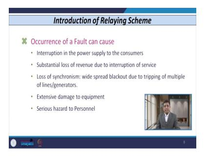
If I list, the first is the interruption of power, of the power supply to the consumer. So, consumers are not able to get the power supply. The second is the substantial loss of revenue due to interruption of services. So, that means, when there is an interruption of power, so that power is not utilized. So, obviously, whatever state electricity board or company is there, they will lose the revenue. The third point that is known as loss of synchronism.
