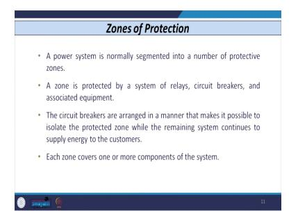
So, these circuit breakers are arranged in number of different manners so that we have the, all the devices which we have discussed in earlier slide, all are protected against all types of fault.
