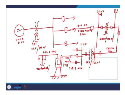
If we consider the major components of power system network, then we know that normally, the power is generated in the power station. The power is generated in the power station at the voltage between 11 kV to 22 kV. So, usually in our country, the power is generated at 11 kV or at the most 13.2 kV, whereas in some other developed countries, the power is generated at voltage 22 kV.
