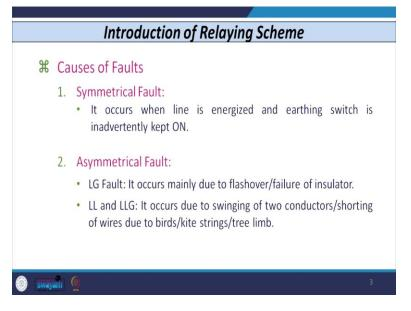
So, line to ground fault usually occurs due to flashover of insulator or sometimes the failure of the insulator.
