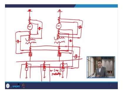
So, for that, if I consider the same diagram, let us say, we have the generator right here, then we have the generating transformer and then we have the breaker along with which is connected to the bus. Same way, let us consider the same on this side also we have the generator, we have the generating transformer and then it is connected to the bus through the circuit breaker. So, these two are the circuit breakers.
