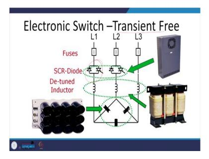
So, this is the way to put it, the electronic transient free. Ultimately you have a thyristors. So that will turn on and turn off thyristors and diode combinations, and you have a inductor and they have a capacitor bank. This is for the electronic switch transient free operation. I request the student to refer to the, my facts devices courses, these entities are been discussed in detail.
