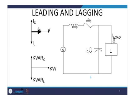
So, for this reason this is we can have a leading and lagging power factor, this is inductor and for this is in you have a capacitor, we can have a load. So, for this reason we require to correct the load and we can have a resonance condition when capacitive VAR and the inductive VAR are matches each other and thus system behaves as a resistive circuit.
