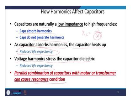
So, what generally we do? How the harmonics affects the capacitor? Capacitors are naturally because you know Xc equal to 1 by omega c. So, higher is the omega, lower is the impedance. The capacitors are naturally a low impedance to high frequencies and thus capacitor absorbs the high frequencies. Capacitor do not generate harmonics. So, there is an advantage of it.
