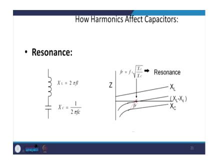
So, for this reason we have to, we know that what is harmonics ultimately for a series harmonics it is  $X_L$  and this is  $X_C$ . Ultimately this is an  $X_C$  and  $X_L$ . So, this will be the natural frequency of oscillations when  $X_L$  equal to  $X_C$ .
