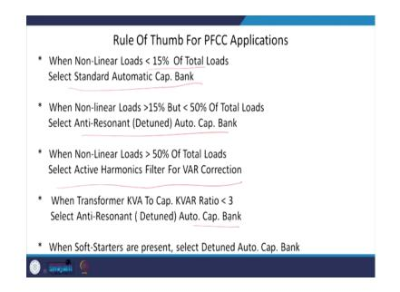
So, role of this, role of thumb of the power factor correction. When non-linear load is less than 15 percent select the standard automatic capacitor, when non-linear load is above 15 percent to 50 percent select the detuned anti resonant capacitor, when load is more than 50 percent select active harmonic filter of the VAR corrections. When transformer KVA or capacitor is around 3 percent select anti-resonant or detuned capacitor, when soft starters are present select detuned auto cap.
