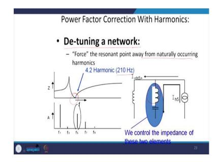
So, for this reason power factor corrections with the harmonic, we are now gradually avoiding and we go for the solutions with the active devices for the STATCOM and other devices. So, we required to de-tune this network. Force the resonance point away from the naturally occurring frequency and we will make it something like 4.2 harmonic for the 50 hertz or 60 hertz depends.
