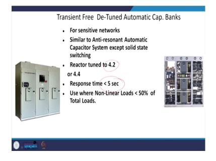
And transient free detuned automatic banks for very sensitive networks, similar to the anti resonant capacitor. It is same. It is been detuned to the harmonic of 4.2 to 4.4 and it has a response time of less than 5 second, where non-linear load is more than 50 percent.
