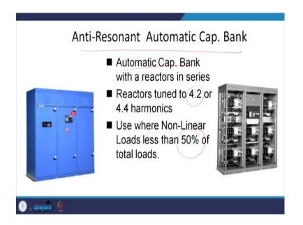
So, for this reason we require the anti-resonant automatic capacitor bank which the C type. This is this pictures courtesy to the same Schneider. The automatic capacitor bank
