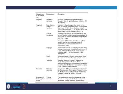
So, first of all it is based on the characteristics of the voltage wave. We can have a power quality in voltage, current as well as the frequencies.
