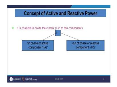
We can then split the current into the in-phase component and the reactive component of it. It is possible to split this into the two components.
