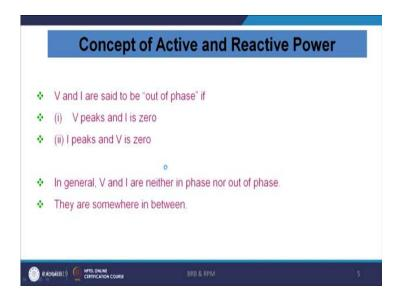
Then, let us see this problem. Voltage and current are said to be out of phase when they are 180 degree of their phase angle. Then when you are charging the battery, voltage and current are in a same phase, through the active filter, once you discharge the battery you can have a 180-degree phase shift when peak voltage, and I is zero, or the I peaks and V is zero. Then in general V and I are neither in a same phase or out of phase. Now they are somewhere in between.
