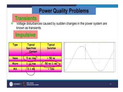
Thereafter let us talk about the transient disturbance caused by the sudden change of the power system and this can be impulsive. Let us see that. These are the ranges of it. The spectral in rise time is 5 nanosecond and typical duration is less than 50. It is micro. This one is the 1 microsecond and typical duration is 50 nanosecond to 1 millisecond and it is 0.1 millisecond. Generally, you have a typical duration of 1 millisecond.
