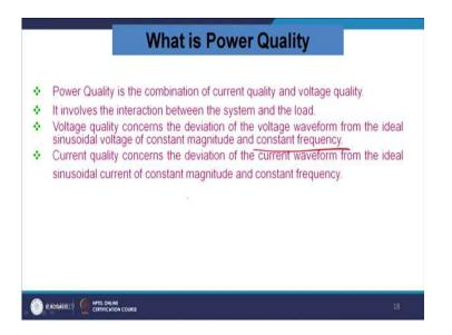
Power quality is a combination of the current and voltage quality and as well as frequency. It involves interaction between the system and the load. Voltage quality concerns the deviation of the voltage waveform from the ideal sinusoidal voltage of constant magnitude and constant frequency. Same way, current quality concerns deviation of the current wave from the ideal sinusoidal constant magnitude and constant frequency.
