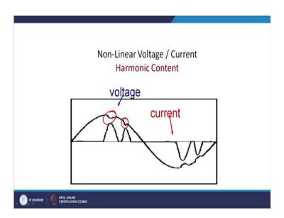
This occurs when the diode bridge rectifier feeding the RC load. The current will have a distortion power factor and due to that current only flows for this duration. There will be a notch in the voltages and current, which will flow only for this duration. This is the non-linear voltage and current with the harmonic.
