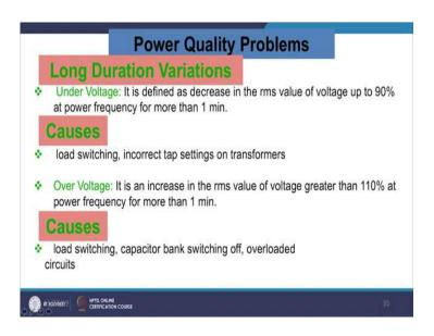
Under voltage: It is defined as decreased in RMS value to 90 percent of the power frequency for more than 1 minute and causes, incorrect setting of the transformer. Over voltage is an increase in the RMS value of the voltage greater than 110 percent of the
