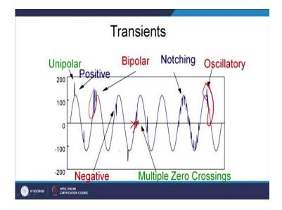
This is the unipolar positive. This spike does not come here and this one is negative and this one is bipolar. You have a double peak. This is notches. Generally, comes due to the thyristor switching and it may be oscillatory. It is coming in a that part of the waveform.
