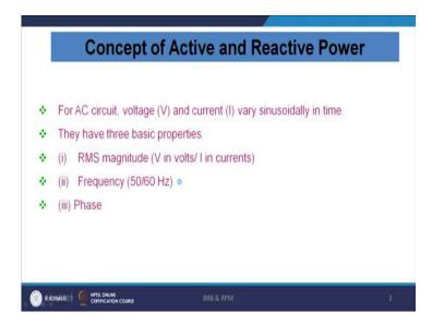
Now, we want to just revisit it for the sake of understanding it. For AC circuit voltage and current are varying sinusoidally, they have the basic properties like RMS voltage and current. Then the frequencies have to be 50 Hertz, 60 Hertz. Then it must have a phase with a desired maintenance ratio. That means it should not have a long phase lead and phase lag.
