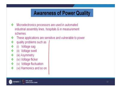
Now, what else? Microelectronics processors are used in automated industry, assemble lines, hospitals. That we have discussed, and we know these are the problems. Power quality have mainly following problems, voltage sag, voltage swell, asymmetry voltage flicker, voltage fluctuations, harmonics and so on.
