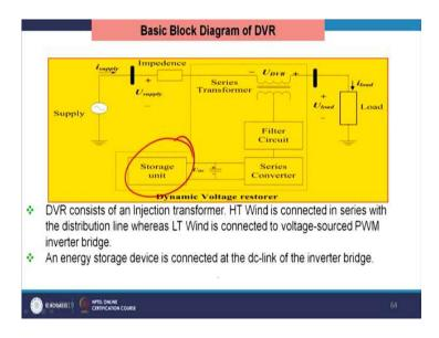
This is the overall basic diagram of the DVR. This is storage unit. This is series converter. This is series filter. In that way, it will compensate the filtering part.
