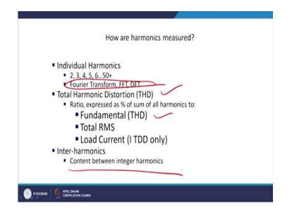
For this reason, we require to define individual harmonic and we know that we can find it with a Fourier Transformation and to measure the harmonic content we have few methods. That is mainly the THD, that is Total Harmonic Distortion and that is a fundamental THD, that is total RMS and the load current RMS and there can be a inter-harmonics. That is another nasty element as well.
