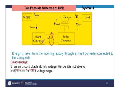
So, this is one of the examples of combining the series and the parallel combination. This is called UPFC. You have a shunt path. It takes the current and it compensates. Again, it has a disadvantage. That is an uncontrollable dc link voltage. Hence it is not able to
