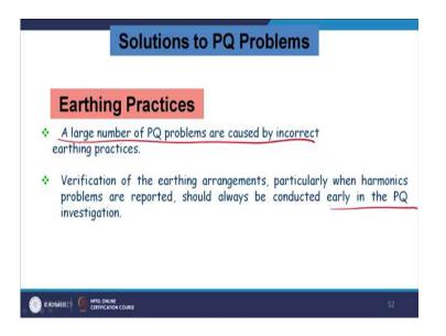
Another solution is good earthing practice. This is also an important entity. The large number of PQ problem is caused by inaccurate or inappropriate earthing. Verification of the earthing arrangement particularly when harmonics problems are reported should always be conducted early at the PQ investigation.
