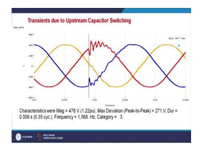
Another example, this is Upstream Capacitor Switching. Till then it was balanced, capacitor of magnitude of 478 volt 1.22 per unit, maximum deviation these and this, duration is 0.006 second, that is 0.3 cycles. Frequency is this much and category? This kind of category you can see that. See here you have undergone the switching and thus it continues for some time and ultimately it deviates. This kind of phenomena are the transient phenomena.
