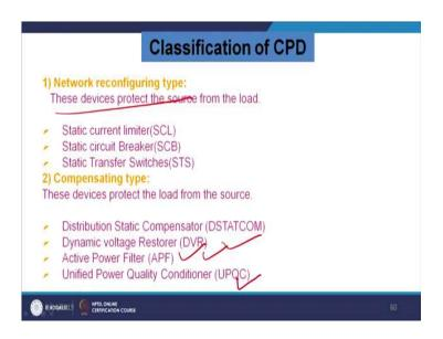
These are the few network configuration type. This type of devices like static current limiter, static circuit breaker, static transfer of switches protects the source from the load. In the compensating type it can be a D-STATCOM. It can be DVR. It can be shunt active power filter. It can be UPQC. So, please recall this. Remember this slide. MCQ question
