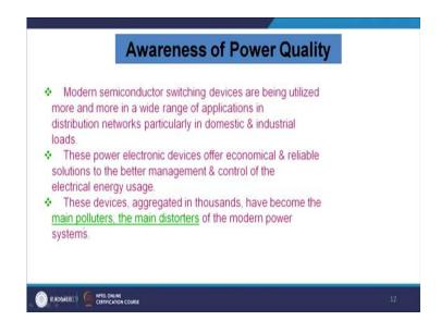
Moreover, modern semiconductor switching devices are being utilized more and more in a wide range of application in a distribution network particularly in domestic and the industrial loads.
