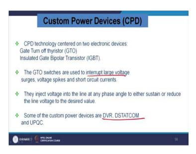
It can be IGBT or the GTO based. The GTO switches are used to interrupt large voltage and current having a higher power rating. But switching frequency is less and some of the custom power devices are DVR, D-STATCOM and UPQC.
