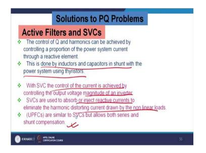
Thereafter we can talk about the solution like Active Filter and SVCs. Control of Q and harmonics can be achieved by controlling the proportion of the power controller. This is
