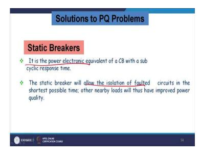
It is the powers electronic circuit breaker. What does it do? This is a static circuit breaker. It can make and break the circuit very fast. The static breaker allows the isolation of the faulted circuits in the shortest possible time and thus, it improves the power quality.
