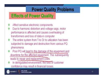
Now, effect of the power quality. We have discussed that thoroughly and so let us take out this point. Poor PQ will lead to the damage of the equipment and downtime for the effected equipment and this subsequently leads to repair and replacement costs. For this reason, we have to take power quality issues quite seriously.
