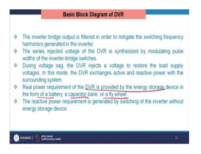
Similarly, we required to provide the real power requirement. It can be provided to the battery, capacitor bank or the fly wheels. The reactive power requirement is generated by the switching of the inverter without requiring any storage device. You can generate it with the help of the angle between the voltage and current.
