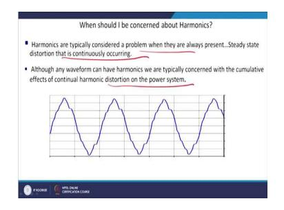
Similarly, the harmonics are typically considered to be a problem when they are always present in a steady state distortion that is continuously occurring. Although any waveform can have harmonics, we are typically concerned with the cumulative effects of continual harmonic distortion on the power system.
