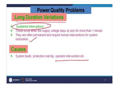
Now, there is a sustained oscillation. So, long duration variations can have a sustained interruption. Those occurs when the supply voltage stays at '0' for the more than 1 minutes. They are often permanent and require human intervention for system restoration. Cause: Maybe system fault, protection mal trip, operation intervention, etc.
