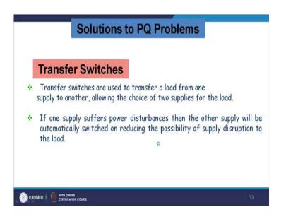
Transfer switches: Transfer switches are used to transfer a load from the supply to another, allowing the choice of two supplies for the load. What do we do generally? We generally put our signal phase load in between line and neutral. We required to put the line and earth.
