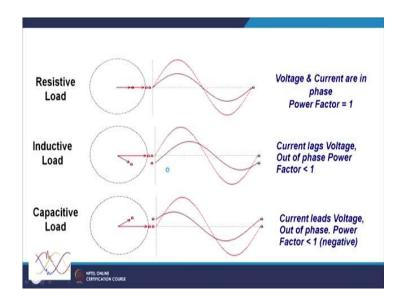
Similarly, for the resistive load with a power factor equal to 1 or unity power factor. This is an inductive load where power factor less than 1 and this one is a capacitive load where it is minus 1.
