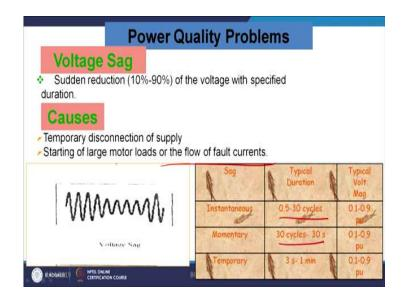
So, what is sag? Sudden reductions of the voltage. We have defined already and cause of the sag is a temporary. This connection of the supply and starting of the large motor load or the fault current. This is the example of the sag. So, instantaneous for 0.5 cycle. We have explained all those things. It is just recapitulations. Momentarily, it is 30 cycle to 30 seconds and temporary it is 3 second to 1 minute.
