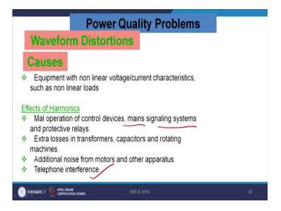
So, cause: definitely, it is the non-linear voltage and current. Effect of the harmonics are malfunction of the control device, mains signal systems, extra losses in transformer, capacitor and the rotating machine, additional noise from the motors and other parameter and telephone interferences.
