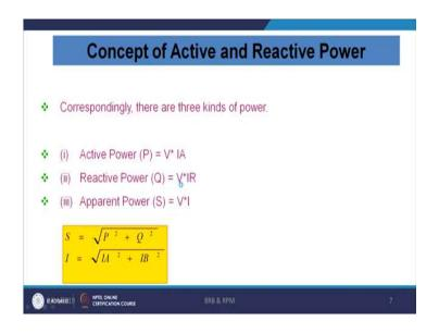
We define as if it is apparent power then it is  $\sqrt{P^2 + Q^2}$ . Then similarly we can split the current. You know that active power equal to  $V \times IA$  and the reactive power equal to  $V \times IR$  and thus the apparent power is  $V \times I$ .
