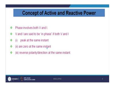
Phase involves both voltage and current then, V and I said to be in a phase. That is what a desired requirement of the power quality. Now, peak at an instant should have a zero crossing at the same instant.
