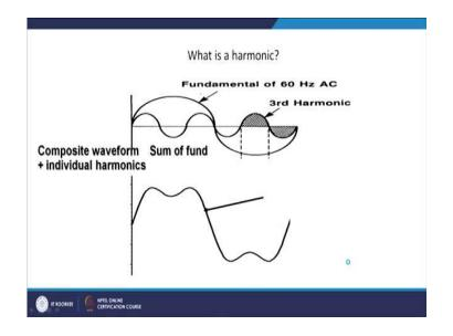
Now, if it is fundamentally 60 hertz. Let us consider that and the 3rd harmonic. Then the composition of the waveform can be this and we call it 3rd harmonic injection. We sometime intentionally do it in drives or it will be like this. It is a contamination if it is available in the waveform.
