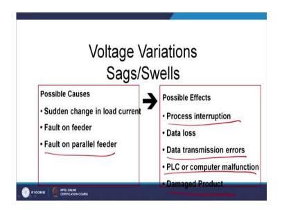
Possible cause of the sag is a sudden change in the load current, fault of the feeder, fault in feeder or fault on the parallel feeder. Possible effect: process of interruption, again data loss, data transmission, PLC computer malfunctions, SCADA may malfunction, damage of the product.
