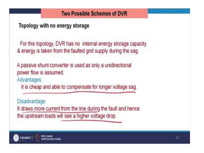
Similarly, there are advantages and disadvantages. Advantage is that it is cheap and able to compensate the longer voltage sag. Disadvantage is, it draws the current from the line during the fault, hence the upstream load sees the higher voltage drop.
