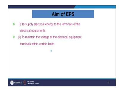
Now aim of electric power supply. That is your utility. To supply electric energy to the terminal of the electric component, that is the role of your grid. Thereafter to maintain the terminal voltage at the electrical equipment within a certain limit is also another aim.
