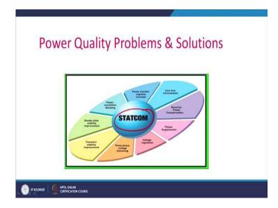
It can be the transient stability, and you know that the STATCOM is a FACTS device that can give you a solution of all those problems like power quality, transfer capacity, oscillation, damping. If you see those power quality problems, we try to find solution through STATCOM or the UPQC. For all the current related problems, we generally use the STATCOM.
