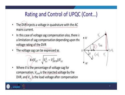
Now let us talk about that. We have discussed the classifications there. Now, let us talk about the rating of this UPQC. So, the DVR injects the voltage in quadrature in the AC mains current and this is the voltage that has been injected in quadrature with the voltage. In quadrature with the current. Pardon me. Ultimately this is the new angle  $\delta$  with the current and it was a previously V<sub>s</sub> and this was a  $\phi$ .
