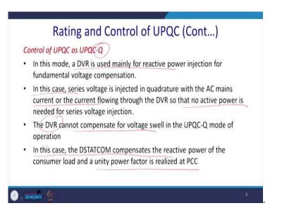
We have discussed this UPQC as UPQC-Q. Just a recall. That in this mode generally, it injects the voltage in quadrature with the current. In this mode DVR is used for reactive power injections for fundamental voltage compensations. In this case, series voltage is injected in quadrature with AC mains. Current flow through the DVR also acts as that and no active power is required.
