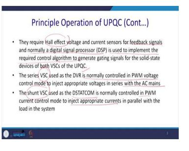
Generally, to sense the current, we have a Hall effect voltage and the current sensors. LEM kind of entities for feedback signals and nowadays we implement in the digital domain. So, it required to be fed in to the ADC s. From ADC it will go into your DSP or FPGA system to generate your control pulses.
