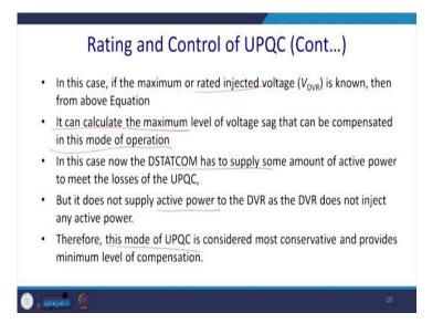
What we can do? In this case the rated injected voltage is known from these above equations. That is fixed because you have chosen that kind of rating. It can calculate the voltage sag and that can be compensated with this mode of operation.
