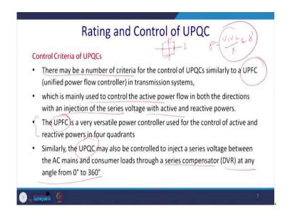
There maybe a number of criteria for the UPQC similar to the UPFC that has been mostly used in the FACTS devices and that is been put into the transmission line. Which is mainly used to control the active power flow because, we deal with the power flow in case of FACTS devices, and we are controlling the quality of the power in case of the UPQC. Mainly used for the controlling the active power flow in both the directions with injections of the series. For the reactive power can also be done.
