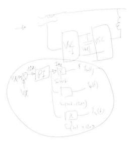
Generally, you have 2 VSC. VSC-1 and VSC-2. This is generally the shunt part and this one is generally the series part. Here this shunt path what happens? You have the  $V_{dc}$ . So,  $V_{dc}$  and you have actual  $V_{dc}$  and from there you will subtract the reference  $V_{dc}$ .
