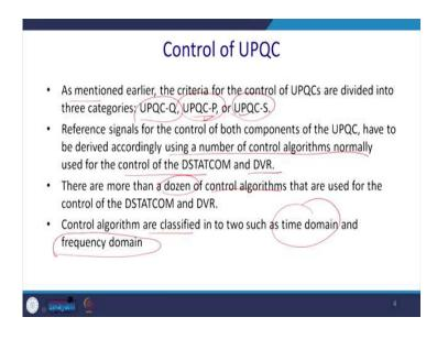
So, we have already discussed that there are different kind of UPQC. That is UPQC-Q. It injects the voltage in quadrature with the current. It injects the voltage. UPQC-P inject the voltage in phase with current and 'UPQC-S' can inject the voltage in appropriate angle or the optimal angle to compensate. So, we have already discussed this method as mentioned earlier the criteria can be UPQC-Q, UPQC-P and UPQC-S.
