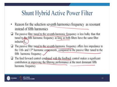
So, reasons for the selections of the seventh harmonic are as follows. These are the passive filter which is tuned to the seventh harmonic frequency (that is what I was telling) and it is less bulky than that tuned to the fifth harmonic as long as both filters have the same inductance  $L_f$ . Because if you put the value the  $L_f$  constant and you change the value of  $C_f$ , then of course, this capacitor will be bulkier
