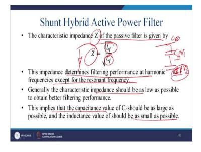
The characteristic impedance Z of the passive filter is given by  $z = \sqrt{\frac{L_f}{c_f}}$ . This is also called the sarge impedance and these we will see. This impedance determines the filtering performance because this will offer at the 50 Hertz. This impedance determines the filtering performance at harmonic frequency except the resonating frequency. So, resonating frequency maybe your seventh harmonic. What will be the impedance offered? That will be in this value.
