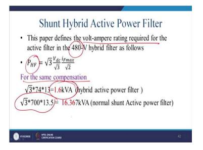
This paper that Akagi has put defines the volt-ampere rating required to be the 480 Volt. That is the standard in Japan. Hybrid power filter as follows. So, that is  $P_{HF}$  that is a power. That is  $P_{HF} = \sqrt{3} \frac{v_{dc}}{\sqrt{3}} \frac{i_{Fmax}}{\sqrt{2}}$ . From there for a same compensation for the hybrid filter you can calculate.
