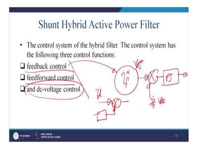
Whether it is an optimal control or whether all are required to be placed or not that is a matter of research, but considering that paper we are going to discuss all this feedback. The control system of the hybrid filter can be feedback control and I will show that. Ultimately as you have seen throughout our discussions you have  $i_f$  or  $i_c^*$ .
