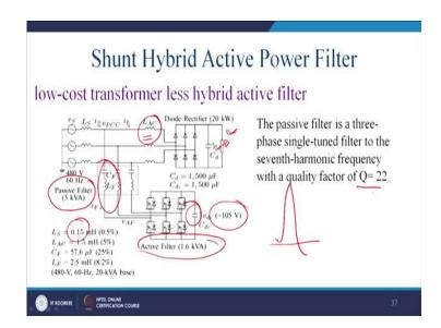
It is a low-cost transformer less Hybrid Active Power Filter and you can see that it is 480 volt 60 Hertz supply and dc bus voltage is maintained to the 105 volt and this is a filter and this has been tuned to the some desire frequency 5th or 7th. It has been tuned to the 7th and the passive filter power rating is 5 kVA and the Diode Rectifier Power rating is 20 kVA.
