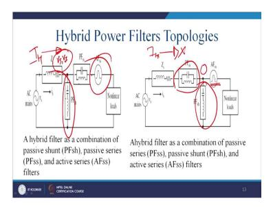
Now, let us see that. Again, in the T network you can add one series passive filter. Sorry. It is not a T network this is a source impedance and you have a combination of the active and passive. You put the shunt first, thereafter series entity and here difference is that you put the series parts then only you put the shunt. What happens then? Generally, since it will block certain amount of the harmonic its rating required is reduced and here it will see the overall rating.
