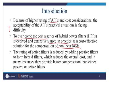
Thus, because of the higher rating active power filter and the cost consideration, the acceptability of this active power filter practical situations is facing difficulty. So, one of the demerits of the active power filter is a higher establishment costs, because you required to put it in a distribution network. If you want to put it into the transmission network, then due to the high cost of the device will come down because of the higher device rating.
