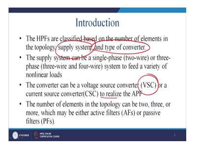
The hybrid power filters are classified based on the number of elements in the topology. Thereafter, it can be based on the supply system. It can be based on the types of the converter. Whether it is a multi level or the two level or you can have a different kind of cascade topology in between. Whether it is even in a multi-level or the diode clamp or the capacitor clamp or the H-bridge or cascade multi-level inverter.
