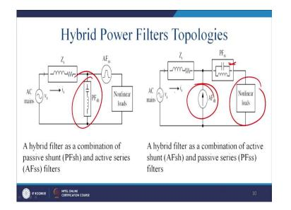
Similarly, we can have a shunt series combination. So, you have a shunt passive filter and series active filter. A hybrid filter is a combination of the passive shunt and the active series combinations. Just reverse and you have a active shunt and the passive series.
