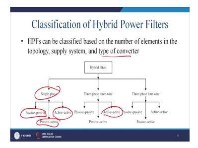
This hybrid power filter can be classified based on the number of elements in the topology. As I discussed earlier, supply system and the types of converter. It can be single-phase and then you can have a single-phase passive-passive. So, this is no longer a power filter. You can have that passive active combination. This is essentially the hybrid entity and also you can have an active-active.
