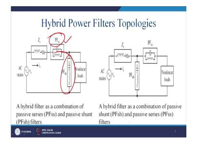
So, let us see that. The hybrid filter is a combination of the passive filter and the passive shunt filter. Then it is called the passive-passive filter. So, you have this one, it is a passive series filter, and this one is your passive shunt filter. This combination, we also call it the hybrid, but it is no longer a power filter though. This combination is called passive-passive filter.
