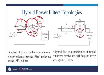
Now, in between you will replace something. Here this is the impedance of the source impedance, that has been coupled or lumped for the short transmission line. Thereafter you have PFss. That is series and now you have active compensation of the series and this is called a hybrid filter, as a combination of the series connection of the passive filters and active series filter.
