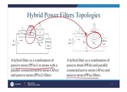
Now, let us see the combinations, that we have already discussed little bit. Thereafter first we have a series compensation for the particular filter. Then we have a series active filter connected parallel to another passive series filter. This is called a hybrid filter, as the combinations of the passive series filter in series with a parallel connected active series.
