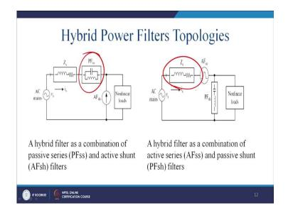
Now, you have AC mains and you can have a series passive filter and shunt active filter. They are connecting like this. This topology is said to be the hybrid filter as a combination of the passive series and the active shunt filter. Similarly, this one is an active series and the passive shunt. This hybrid filter is a combination of the active series and the passive shunt. All the permutation and combinations is possible here.
