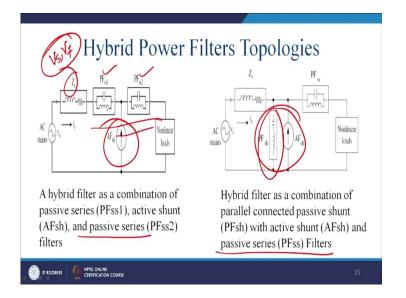
Now, similarly you can have a shunt solution. This is your series passive filter and you have an active shunt solution and that is also possible for the current harmonic mitigations. Hybrid filter as combinations of the passive series and the active shunt, and the passive series combination has been shown. Thereafter you have hybrid filter as a combination of the parallel connected passive shunt with active shunt and the passive series has been shown.
