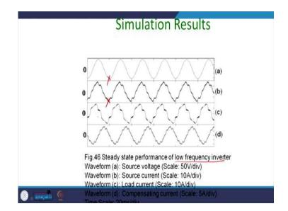
So, now let us come to some simulations and the experimental results. Now, this is a steady state operation of the low frequency inverter. Here low frequency inverter essentially is not operated for the reactive power compensation or the unbalanced compensation. It is not meant for the harmonic composition and for this reason you can see that. This is a source voltage and the source current and the load current and the compensating current.
