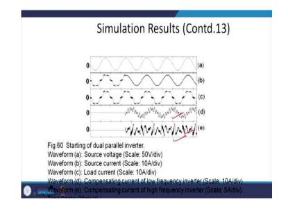
Now I just show both when high frequency and the low frequency are being operated. This is the low frequency harmonic and this is the high frequency harmonic and you can see that. This current is sinusoidal with a unity power factor. Where this injects harmonic and where this injects the reactive power and thus you have segregated the reactive power, as well as this active power.
