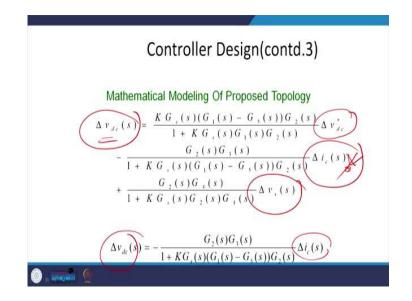
After perturbing, you get a  $v_{dc}$ . Essentially since the DC bus voltage is very low sudden change of the load on the source disturbance can overthrow a DC bus voltage into the zone of the instability. For this reason, maintaining the DC bus voltage is a main challenge here. It was the proper functioning of this shunt active power filter.
