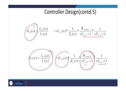
So, it is  $G_6(s) = \frac{I_{F1}(s)}{I_s(s)}$ . Refer to the previous slide. It is  $G_{11}$  equal to  $G_{11}$  into one by  $Z_1(s)$  into that is K pwm into this one.  $G_7$ , essentially it is  $\frac{I_{F2}(s)}{I_s(s)}$ . Here,  $Z_2$  is a impedance. Basically, it gives a switching frequency. So, it did not. Then it will be e to the power something. There is a delay. These entities, then this is equal to delay. This is the switching frequency of this another transformer.
