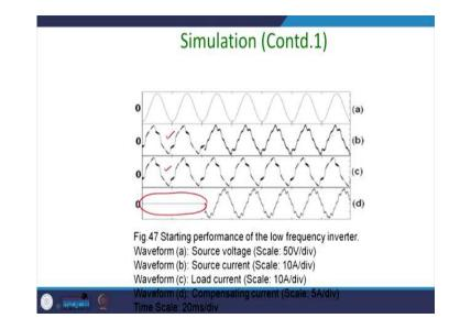
Now this was the load current and this was a source current and now at this moment, you start your low frequency inverter and you can see that its '0' crossing matches or the peak matches and thus it is a unity power factor. But the it is corrupted with harmonics. So, harmonic compensation has not been used here.
