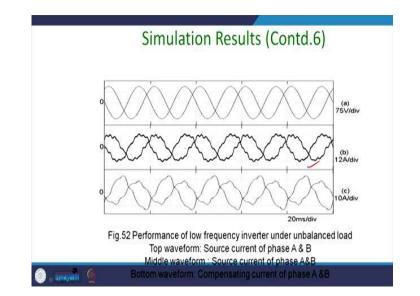
Now, here you can see. It is quite interesting. This is a voltage and current. The load is unbalanced. Source current has got harmonic because of the absence of the harmonic compensation but the source current is balanced. Just it contained the harmonic.
