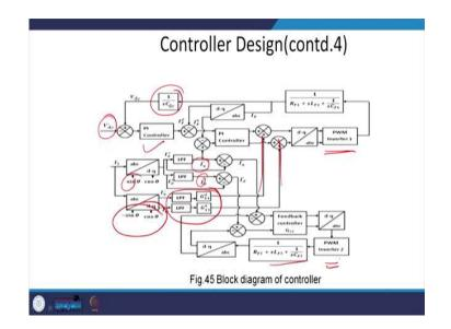
This is the overall block diagram of this control and  $v_{dc}$  is the reference. There after you have a  $V_{dc}^*$ . Thereafter the PI controller. You have  $\frac{1}{sC_{dc}}$ . Then you subtract these two entities in a 'dq' frame and here you have RF plus L<sub>F</sub> plus C<sub>F</sub> also. This is for the first filter and your PI controller and from the PI controller, you can have 'abc' to 'dq' frame. You feed it to the PWM block.
