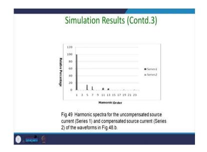
Then this is the harmonic spectrum of it and you can see that there the is a harmonic spectrum is quite good. This black one is essentially the load current or the uncompensated source current and the gray one is the source current.
