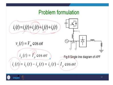
So, load current. It can be expanded with because you have taken a sample and this sample may have a quantization error and due to that you may have some DC component or you may be triggering the thyristors. If thyristors for the non-linear load and if their angle is little different then alpha is required to be compensated. So, for the small interval of time this DC component may come. Ultimately it will be adjusted.
