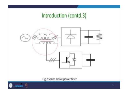
Another can be your shunt series active power filter where you inject the current. Thereafter what happened? You get the voltage sag or swell. It will be unique, injecting voltage in phase. This aspect, we have covered in the series portion of the UPQC in detail and thus our lecture will be concentrating mainly on the shunt, but as the topology concerns.
