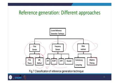
So, reference generation technique can be broadly classified into the time domain. One is the PQ theory: That is proposed by the father of this shunt active power filter, professor Akagi and SRF method: SRF method essentially was derived from the vector control of the induction machine drive. It is quite old method, but it has been taken from there.
