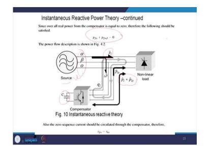
So, this is the pictorial diagram of the shunt active power filter in the domain of the power quality. We know that this is '0' as per the shunt active power filter. So, this is the figure we have considered and here we represent it into the ' $\alpha\beta$ ' frame instead of the source current 'abc'.
