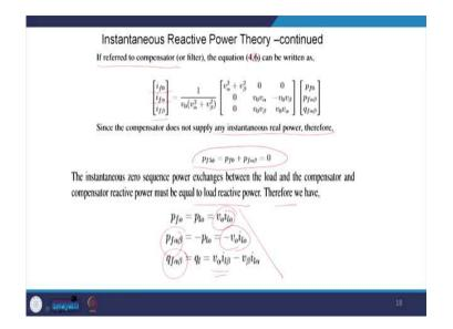
So, based on that we refer the compensator of the filter and this can be written as follows. This is the ' $\alpha\beta$ ', this is the component of this active power filter. This will be the zero-sequence component, this will be the ' $\alpha$  &  $\beta$ ' component of the shunt active power filter. That will make that instantaneous real power to be '0'.
