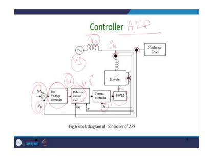
So, ultimately this is a control block diagram of active power filter. So, you have  $V_S$  here and you have  $L_S$  here  $R_S$  has been neglected. You, will sense this load current before the point of common coupling, after this point of common coupling. This point is called PCC. So, you will go to the reference generation calculation and then you will sense this dc bus voltage of the shunt active power filter inverter and that will be there and you require to maintain the DC bus voltage.
