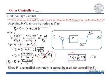
So, let us see that this is an AC voltage control and if distributed network is a weak network and the AC voltage has to be regulated by the voltage source controller, then instead of the grid, it is a rigid body. So, we have to apply the KVL and ultimately you have the current that is basically your voltage by the apparent power.
