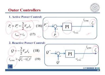
So, there is the outer controller. This was the inner controller and this will control the your active power. You know that active power P<sub>c</sub>. We neglect the losses that is something we require to if you do total modeling then you require to take the losses. So, it is  $P_c' = \frac{3}{2}V_{gd}i_d$ .
