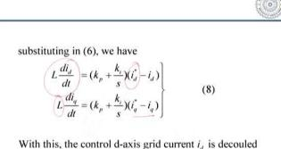
With this, the control d-axis grid current  $i_d$  is decouled with  $i_q$  and vice-versa.
