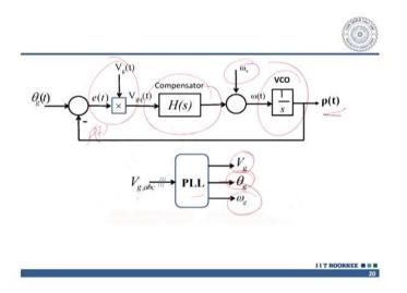
So, the error is e(t). So, that is the  $\rho(t)$ , e(t), you multiply with  $V_g(t)$  that gives you the q axis voltage and you have got a compensator. That is basically maps the voltage into the frequency. So, that error represents the voltage. You subtract with the unit voltage template and you feed it to the integrator. Because I told you that if you integrate, ultimately you get the  $\Theta$ .
