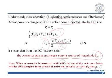
So, what we can say that under steady state conditions and we assume that these losses are neglected, semiconductor losses are neglected, filter losses are neglected. So, active power exchange at PCC that his point of common coupling equal to active power injected into the DC side of the PCC and thus  $\frac{3}{2}(V_{gd}i_d + V_{gq}i_q) = V_{dc}I_{dc}$  need to me maintained. Thus, I<sub>dc</sub> value should be equal to  $\frac{3}{2}\frac{(V_{gd}i_d + V_{gq}i_q)}{V_{dc}}$ .
