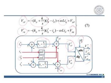
So, how this block diagram has been represented? It is a voltage. So,  $V_{cd} = -\left(k_p + \frac{k_i}{s}\right)(i_d^* - i_d) + \omega Li_q + V_{gd}$ .
