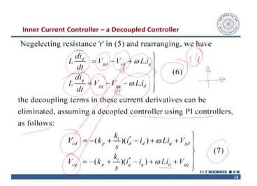
So, what happens? So, you got L di/dt and there is little simplification just  $r \times i_d$  is actually omitted, considering that resistance part is quite less. So, you got V<sub>d</sub> minus the d axis component of this converter voltage plus  $\omega L i_q$ . Similarly, you have the q axis
