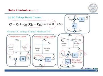
So, let us recap what we have said. This is called the voltage droop control. Sometime it is very much useful because once you find that voltage is drooping that is not applicable only on power quality issues, but also in case of the distribution system, especially we are talking about DC micro grid. They are featured in a long way. So,  $P_c^* - P_c + R_{DC}(V_{dc}^* - V_{dc}) = 0$ . Then you say that you are maintaining a constant voltage.
