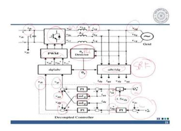
So, let us see that overall block diagram of it and it is applicable for D-STATCOM, it is applicable for the active power filter, it is applicable for or active rectifier and also solar inverter in case of the micro grid. So, this all can be tackled into the single block diagram and this mode of control is called a SRF mode. So, ultimately if you have a real source then i<sub>dc</sub> will be sinking. So, assume that you got a real source and you can feed the power to the grid.
