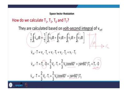
So, now question is how to compute or calculate the value of this times  $T_1$ ,  $T_2$ ,  $T_0$  and the  $T_7$ ? Generally,  $T_0$  and the  $T_7$  are having a same value and just put at the end or at the beginning of the switching cycle. So, if you do this voltage and the time integration of the voltage that is necessarily flux and you divide it by T, then it will raise the voltage only.
