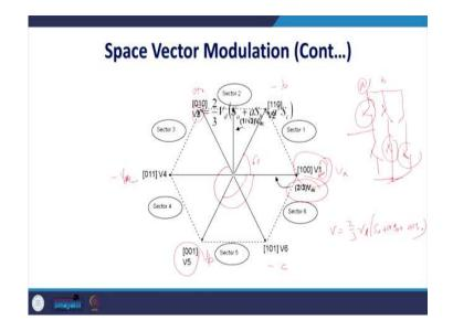
So, the switching logic comes into the picture. Thus, what you have is only this value. Thus, it is  $\frac{2}{3}V_{dc}(S_a + aS_b + a^2S_c)$ . Now, this is the typical two-level phase vector representations. First of all, if you want to have this vector which is said to be 'a' that means that is in upper leg of 'a'. It is closed and it is opened and for the lower two leg this is open and this one is closed. Let us say this is 'a', and this is 'b', and this is 'c'.
