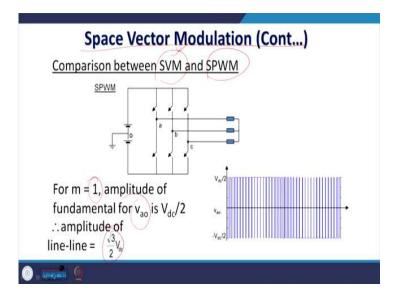
So, this is the way to calculate the times for the two-level space vector modulation. Now, we required to understand that what is the benefit of it or a comparisons of the sin triangle PWM with the space vector modulations. One aspect is that we just say one thing that sin PWM is simple to implement. We can implement this sin triangle PWM very easily.
