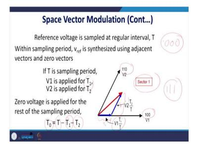
Now, we require to generate the switching logic for this inverter, so that we can accurately generate those reference. It is in a first sector and so, the switching will be  $[1 \ 0 \ 0]$  that mean in upper switch 'a' leg is short and minus 'b' and minus 'c' is short and in this case you know this is a one bit change. Upper legs are short and the 'c' phase is short.
