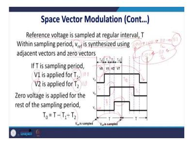
So, as I told you that you are generating the clock pulses from DSP or FPGA, and for this reason the reference voltage sample at a regular interval that is T with a sampling period of  $V_{ref}$ . It is synthesized with adjusting vectors and the zero vectors. If T is a sampling period,  $V_1$  is applied for the time  $T_1$ , and  $V_2$  is applied for the time  $T_2$ , and zero voltage is applied as I told you for the rest of the sampling period that is equal to T in between this.
