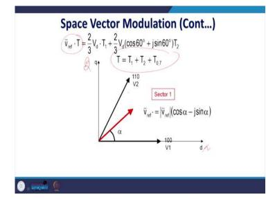
So, what happens now? We can rewrite these equations, where  $T = T_1 + T_2 + T_{0,7}$  and we can rewrite this like this. So, this is the angle alpha ultimately  $\bar{V}_{ref} = |\bar{V}_{ref}|(\cos \alpha + j\sin \alpha)$  you can equate them in alpha beta axis and later if you rotate this by the synchronous frame, this alpha beta become dq frame of reference.
