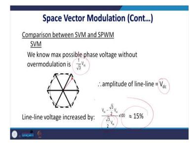
An amplitude of line-to-line voltage can be up to  $V_{dc}$ . Thus straight away you know you can see that the line-to-line voltage in case of the space vector modulations is  $\frac{V_{dc} - \frac{\sqrt{3}}{2}V_{dc}}{\frac{\sqrt{3}}{2}V_{dc}} \times 100 = 15\%$  hence 15 percent increased in the utilizations in the line-to-line voltage for the output of the inverter, and thus we can transform into the better utilization of the dc bus voltage. So, this is the one opportunity of it.
