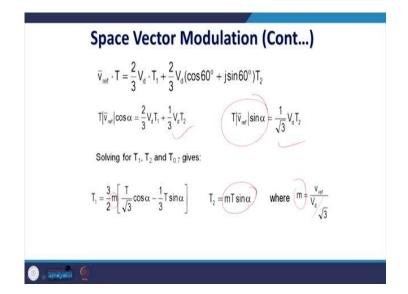
Thus, splitting in x and y axis which is equivalent to the alpha and beta. We can write that is  $v_{ref}$  into T like this. So, equating the real and the imaginary part, we can write like this you know T.  $|\bar{V}_{ref}| \cos \alpha = \frac{2}{3}V_d$ .  $T_1 + \frac{1}{3}V_dT_2$ . Similarly, T.  $|\bar{V}_{ref}| \sin \alpha = \frac{1}{\sqrt{3}}V_dT_2$ . This is the equation.
