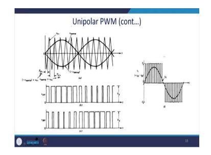
Thus, you require two modulating waveform and one carrier waveform. This is a  $V_{control}$  and this is minus  $V_{control}$ , this is for leg A and this is for leg B. So, this will be the waveform pattern for leg A and this will be a waveform pattern for the leg B. You sum it up. You get this voltage. You can see that there are no negative pulses in positive half cycle.
