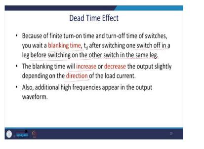
Another important issue we required to discuss is students are required to implement these active rectifier power quality condition as a hardware in master's level or the B Tech level. We required to deal with the switches. Because of the finite turn on and turn off time of the switches you wait for the blanking time.
