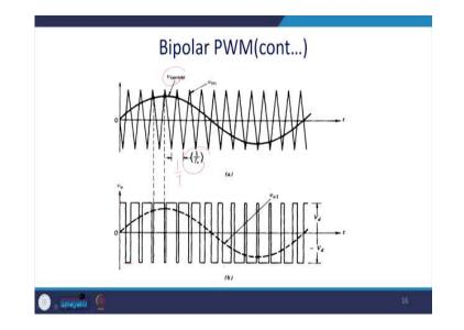
So, how does it work? This is the part of the 1/f, that is the T. It may be 1 kilo hertz that is 1 millisecond and you have a V<sub>control</sub> and the V<sub>tri</sub> you can see that this voltage positive as well as negative. For this reason, we call this as bipolar PWM. So, voltage stress is quite high, because it is switching in half cycle positive to negative. But difference of the voltage will come and that will be effectively positive half of the sine wave.
