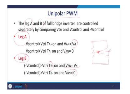
So, let us come to the unipolar PWM. So, logic will be a little different here and we required to generate the sine or the modulating wave and negative of the modulating wave. Not the 'NOT' gate which we have used in case of the bipolar PWM.
