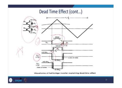
This is some example of this dead time effect and you have to give a little time for the legs so that short does not occurs. You have studied, you know effect of the source inductance in basic power electronics, where, you have essentially overlap angle between the two thyristors that is called ' $\mu$ ' and in between there is no power being transferred because of the shorting of these thyristors.
