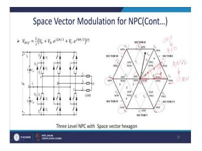
Now, see that I just represent it here, diode clamp three level inverter for sake of simplicity you can extend this to any level. So, this is the '0' and you can have this PPP, NNN, 0 0 0 as a 0 vector. Thereafter  $V_1$  this is the magnitude. Look this magnitude is essentially  $2V_{dc}/3$  and essentially you can have a half voltage vector. You can see the magnitude of it. So, from the triangle you can see that this angle value.
