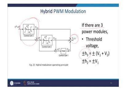
Now, you see that the hybrid modulation technique. This is the one control cell and ultimately you generate the voltage  $V_3$  and it will come out here. So, this one will be fed here. This is another control cell then this will be feeding here ultimately you will get a value  $v_{aN}$ .
