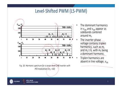
And ultimately this is the case. For the level shift at one (Please recall we have a phase shifted on one also) the ratio we assume that 60 and for this reason we can see that this is the phase voltage versus V<sub>d</sub> and you have a fundamental apart from that you have a 60th harmonic and there after a  $m_f$  + 6 and  $m_f$  - 6 and so, on and ultimately you get around 18 percent THD.
