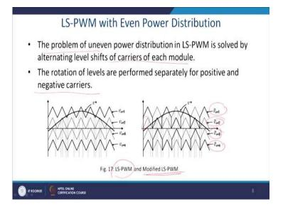
That is what I was discussing right now level shifted PWM and this one is a modified level shifted PWM. Let us see what is the difference between these two. The problem of the uneven power distributions in level shifted PWM is solved by alternating level shifted carrier of each module.
