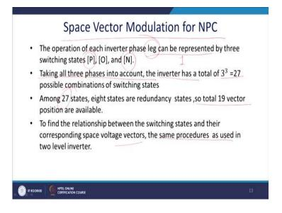
Now, let us come to the space vector modulation technique. I have discussed the space vector modulation technique for this two-level inverter and that has been extended to the three-level inverter. So, basic assumption is same. So, we require to find it out since we managed with 1 and 0 in case of the two level. But we required to since there is a three level, we shall state the concept P for the positive, 0 or O for the middle level and the 'N' for the lower level.
