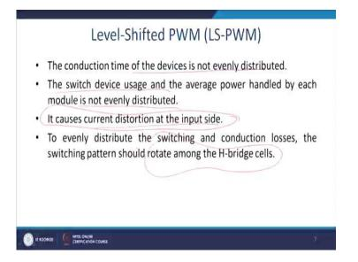
Few more observations. The conduction time of this devices not evenly distributed. As you have seen and due to that what happened? The conduction losses of the different cascade H-bridge multi level inverter, cascade entities, cascade H-bridge will be different. So, losses are not equally placed, so there were local hotspots.
