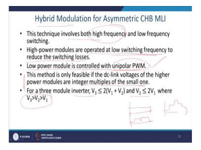
So, what we can conclude from the hybrid modulation asymmetric multi-level inverter? This technique involved both high frequency and the low frequency switching. The power modules are operated at a low frequency to reduce the switching losses.
