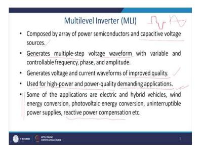
This is an multi-level inverter and it is essentially composed of array of the power semiconductor and the capacitor voltage sources. Array of power semiconductor is generally the diode clamp multi-level inverter. We shall see little later and the capacitor voltage sources are the capacitor come multi level inverter. What does it do?
