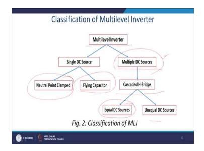
So, this is the classification of the multi level inverter. One it is a multi level inverter, so you can have a single DC source. These are mainly classified into the neutral clamp that is in a diode clamp and this is a flying capacitor. Also, it required a multiple DC source.
