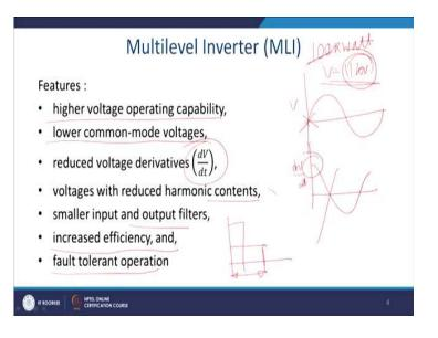
So, features: higher voltage operating capability. It is because of the stress across the switch it has been lowered. Lower common mode voltage. We shall see that. Common mode voltage is between these two legs. This is a differential voltage and another is to with the central of the capacitor.
