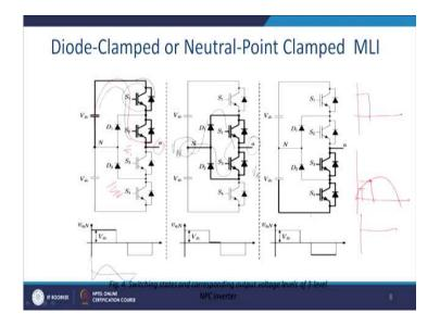
So, let us see that how does it work? That I try to explain here, that you know when we want that it will get  $V_{dc}$ , then upper two switches  $S_1$  and  $S_2$  will be closed or you can write  $S_3$  as  $S_1$  prime and  $S_4$  as  $S_2$  prime. For this diode clamp MLI you want this voltage as I told you. You close these two switches.
