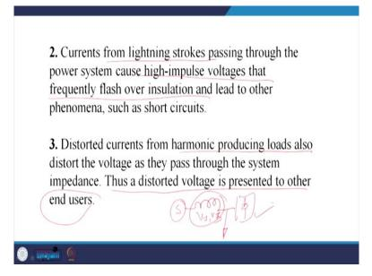
Current from the lighting strokes passing through the power system causes high impulse of the voltages that frequently flash over the insulations and lead to the other phenomena, such as short circuits or trip of the breaker. Distorted currents from the harmonic producing load also distorts the voltage.
