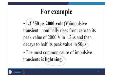
For example, so 1.2 into 50 microsecond and that last for the amplitude of 2,000 volt. Impulsive transient normally rises from Zero to its peak value of 2,000 volt in 1.2 microsecond and then decays half of its peak value in 50 microseconds. If you write like this, it tells like that and most common cause of the impulsive transient is the lighting. So, this is the way we will write.
