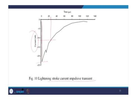
So, this is the example of the lighting stroke current impulsive transient. So, it can be either of the polarity. So, you can see that it goes to some voltage or current in this case this is a current in kilo ampere. So, this is the rise time and you can calculate, what is the rise time here and you have to calculate. So, let's say it is around time-24µs and current-12kA. So, what is the time here? So, this is a way it is generally classified.
