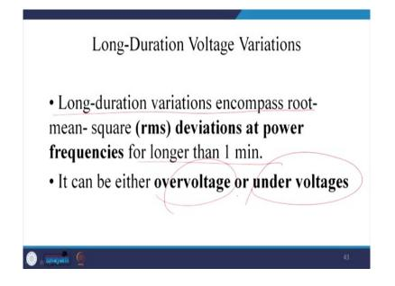
So, there after long duration voltage variations: so, these are the sags and the swells. Long duration voltage variation encompasses root-mean-square deviation at power frequencies for longer than one minute. We will consider that as a long duration voltage variation. It can be either over voltage or it can either as under voltage and it is a sustained duration and that is more than one minute.
