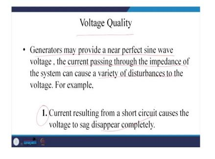
So, what is the voltage part of the power quality? The generator may provide a near perfect sine wave very close to sine wave voltage. The current passing through the impedance of the system can cause variety of disturbances in the voltage. For example, current resulting from the short circuit causes the voltage to sag and disappear completely.
