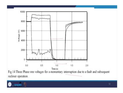
So, here this is the voltage and all of a sudden it has been dropped for interruption again it has picked up this. The 3-phase RMS voltages for a momentary interruption due to a fault at a subsequent recloser operation and thus this is the duration of the interruption.
