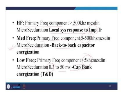
So, oscillatory transient: for example, if it is high frequency, primary frequency component will be 500 kilo Hertz micro second duration. So, local system response to Imp Tr. Med frequency primary frequency component will be in the range of less than 500 kilo Hertz to 5 kilo Hertz. So, microsecond duration back to back capacitor energization, that may cause this
