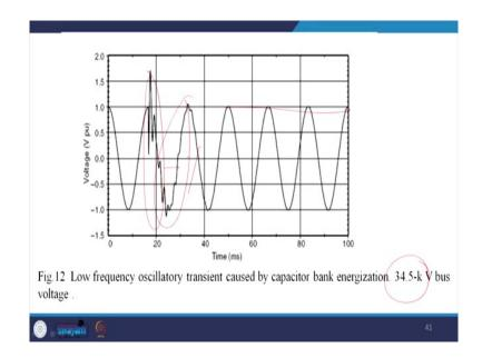
Now, this is the example of the low frequency oscillatory transient caused by the capacitor bank energization that is 35.4 kilo bus voltage. You can see that this voltage is distorted. Thereafter this voltage is distorted. Thereafter again it comes to the smooth oscillatory thing. So, this is a problem, till this point peak of this voltage to this point had a transitory oscillation because of the switching of the capacitor bank.
