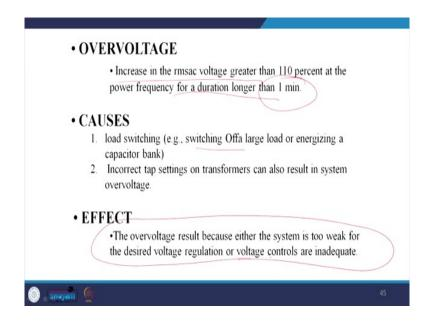
So, first define it, over voltage increases the RMS ac voltage greater than 110 percent at the power frequency for a duration longer than 1 minute. Cause: it may be due to the switching example switching of a large load or energizing a capacitor bank, incorrect tap settings of a transformer can also result in system over voltage. Effect, over voltage results because either the system is too weak for desired voltage regulation or voltage controls are inadequate. So, this is the reasons of it.
