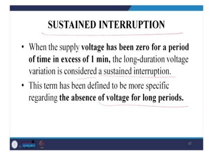
So, another way is a power cut, that is called sustained interruption. When power supply voltage has been zero for a period of time excess of one minute, the long duration voltage variation is considered a sustained interruption. This term has been defined to be more specific regarding the absence of voltage for long periods.
