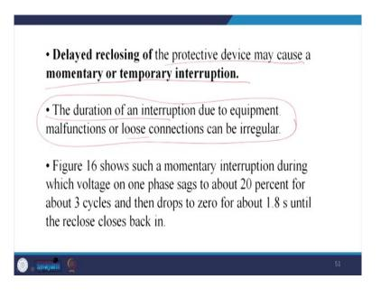
So, delay of reclosing the protecting device may cause the momentarily or the temporary interruption. So, that is also a feasible entity. The durations of an interruptions due to the equipments malfunctions or loose connections can be the irregular pattern of the interruption can also be possible. This you can see very frequent and figure 16 shows the momentary interruption that I am showing here.
