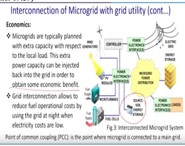
So interconnection of the microgrid with utility grid. One reason is the economics. Microgrids are typically planned. So for this you can see that you know these are wind generations. This is a PV module. This is the microturbine and you may have a fuel cell and ultimately power electronics comes into the pictures and this is the battery and this is a microgrid distributions.
