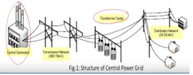
So structure of the conventional central power grid can be described below as the conventional power grid is an interconnected network for delivering electricity from supply to the consumers consisting of generating stations that produce electrical power, high voltage transmission lines that carry power from distant sources to the demand centers and has distribution line that connect individual customers.
