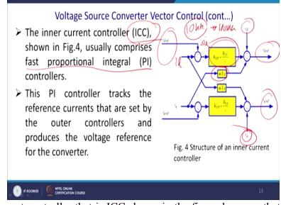
Now the inner current controller that is ICC shown in the figure here see that how does it work and it has a cross relations. So, you have ID reference and this is essentially is a voltages in DQ frame and ultimately you have to you have to compare with other voltages. So, what happened here you know this point is your ID and this is your ID ref and thus you get the Delta ID and that you feed it to the PI controller.
