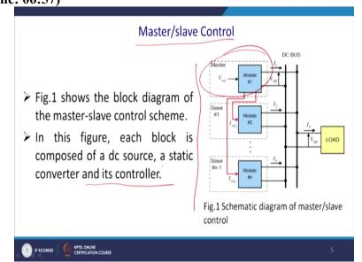
Now master slave control will be almost the same thing what we have discussed in our previous class in case the AC micro-grid. So, master slave control essentially you have a DC bus and this is the master. Task of the master to set the DC bus voltage according to the load condition if it is 48 volt they need to have a little bit of tolerance so load is little bit increasing it can push up it can either take down the voltage little bit low every 46 volt or some amount of tolerance.
