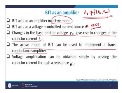
And therefore what we have learned just now therefore is that a change in the base emitter voltage which is this one gives rise to a change in the collector current  $i_c$ . I think this has been already discussed to a larger extent so for example if you are using a silicon transistor and your  $V_{BE}$  is less than 0.7 you can be amply sure that the emitter base junction is cut-off and therefore there is no current appreciable amount of current flowing through the emitter base junction.
