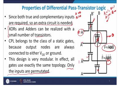
With this knowledge or with this idea, let me come to the next one that let me take up the properties of differential pass transistor logic and let us see how it works out. So since both true and complementary inputs are required, so extra circuitry is needed just to complement the signal. So I require an extra static inverter to complement the signals. Of course, XORs and Adders can be realized using small transistors, one example is given here where XOR and XNOR are designed.
