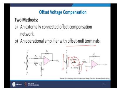
We come to the offset compensation voltage compensation, so there are two methods by which you can compensate the offset voltages and these two compensations are externally compensation, externally connected of set compensation network and with the null offset terminals. So we would not go into the details but I will give you an idea how it works out in a very simple manner. So you see I have  $V_i$  here which I am giving. I also have a 100 ohm  $R_1$  and 100 kilo ohm here.
