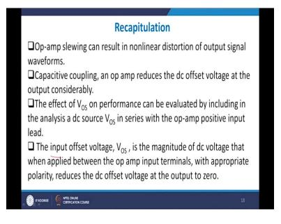
So let me recapitulate what we did, we were actually looking into an op-amp slewing action. What is the meaning of slew right and what is slew rate, slew rate limited operation? What is a DC offset voltage right and how do you define DC offset voltages? What is the meaning of saturation, operational amplifier saturation? What is the meaning of input offset voltage  $V_{os}$ ?
