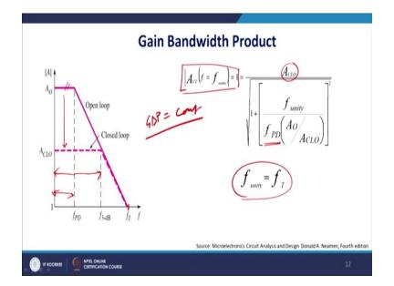
Now gain bandwidth product is given by closed loop gain if you look very carefully, unity  $f_T$ ,  $f_T$  is unity gain bandwidth is given by CLO which means that the closed loop circuitry 1 plus f unity; f unity is  $f_T$  divided by  $f_{PD}$ ,  $f_{PD}$  is basically my 3dB into  $A_{OL}$  by  $A_{CLO}$ . And therefore I get f  $_T$  equals to, so f unity is equals to  $f_T$ , provided I get  $A_0$  by  $A_{CLO}$  very high, right.
