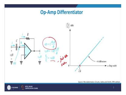
Let me come to the differentiator part, Op-Amp differentiator and if you see differentiator we have just switched to the place of capacitor and register here, so capacitor is here and register is here, so I get i equals to  $C(dV_i/dt)$  differential equation. So, if I take differential signal and
