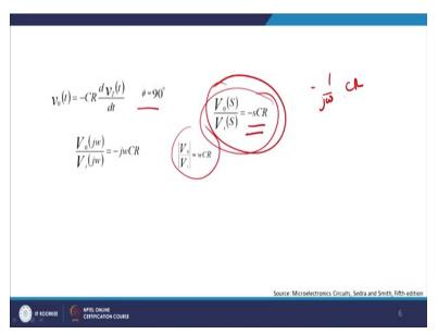
Exactly, the same thing as I did it in the previous turn,  $\phi$  equals to 90 degree, I get output voltage V<sub>0</sub> by V<sub>R</sub> equals to minus s times CR, right. So, minus S is minus 1 by j $\omega$  into C into R, right and that what gives you the value of your output voltage.
