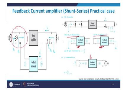
Let us look at the feedback current amplifier. It is basically a shunt series application so I have got a shunt here, right? And I have got the series application here. So, I get  $R_s$  is parallel to  $R_{11}$  and I get  $R_{12}$  here in this place multiplied by  $R_L$ , right? And this is output impedance I have shorted it because any output impedance to confuse at this point of time.
