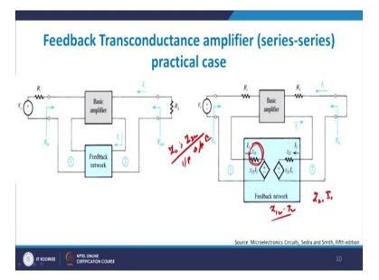
Now, let me come to a practical case of series series amplifier and you see here that I have broken down the feedback network into  $Z_{11}$ . So, it is basically a Z parameter which is available to me. So,  $Z_{11}$  and  $Z_{22}$  are basically the resistance input resistance and output resistance offered to the device and I get  $Z_{21}$  I<sub>1</sub>and  $Z_{12} * I_2$ . So, you see your feedback network is changing.
