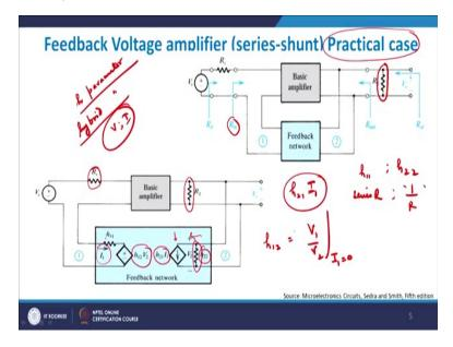
What is  $h_{12}$  therefore?  $h_{12}$  is nothing but if you look very carefully  $h_{12}$  I am referring to as  $V_1/V_2$  with  $I_1$  equals to 0.  $I_1$  is open  $I_1$  is equal to 0.  $I_1$  0 primarily means that you are opening the input site and that is pretty important that you are opening the input site. So, the input site is open. In
