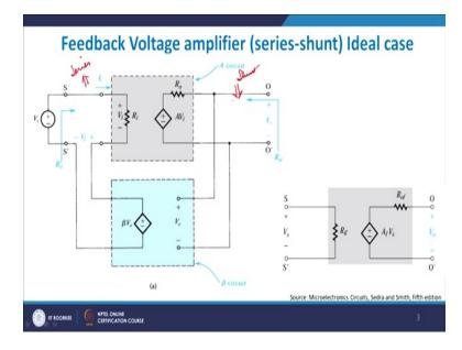
Why because if you look very carefully then you will see that that this is basically a series addition here. And therefore, the impedance levels will go high. This is a shunt or a parallel addition here and therefore, impedance is lower down. That takes cares of approximately all the understanding here.
