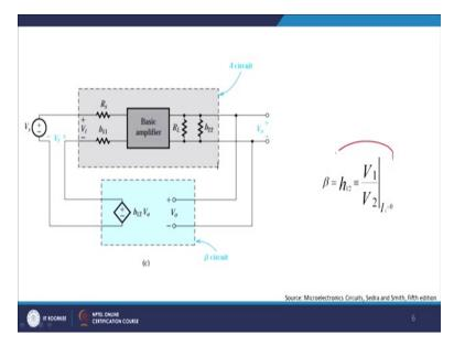
With this knowledge you can safely write down  $h_{21}$  is nothing but  $V_1 / V_2$  with  $I_1$  equals to 0.
