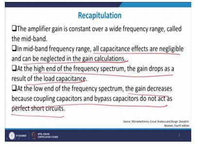
We come to the, let me recapitulate therefore, generally amplifier gain is constant somewhere in the mid frequency band. At very high and low frequencies the gains starts to fall down for high frequencies fall down with increase in frequency. At low frequency it falls down with decrease in frequency. The mid-band frequencies are all the constant and in that case all the capacitive effects are negligible and can be neglected in gain calculation.
