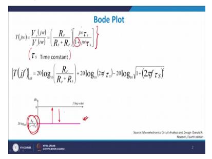
As you can see here the same graph which I was plotting for you, I got this as my frequency scale, this is 20 log  $R_P$ , assuming that  $R_P$  and  $R_S$  is very small, I can, this could be safely assumed to be almost equals to 0, if not it will be lower than this because obviously this quantity will always be smaller than 1 and therefore this will be slightly less than zero.
