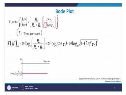
So if you remember yesterday we tried to find out this TJ of J omega and we found out to be  $R_P$  upon R s plus  $R_P$  into j of omega tau s upon 1 plus j omega tau s where tau s is defined basically the time constant of the circuitry and omega is the frequency which is you get and which is equals to 2 Pi f.
