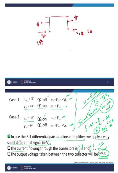
Let us suppose, that I have got two arms here right and these two arms are going on here, in this arm I increase the base voltage  $V_B$  and in this arm I reduce the base voltage  $V_B$ , so if I increase it the current becomes larger, right the current increases, as the current increases this voltage will drop down here. Similarly, when the base voltage reduces the current reduces and therefore the voltage at this point actually increases.
