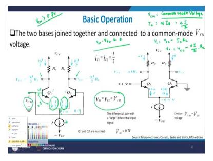
So, this is the basic differential amplifier this thing diagram. Let me see, what happens if we apply the same potential to the base of Q 1 and Q 2, so what I have done? I have simply applied a positive bias here and the same potential is applied to the base terminal of Q 2 and this is basically known as a common mode  $V_{CM}$ ,  $V_{CM}$  is referred to as a common mode voltage, right.
