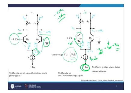
Now, let us see, what is the allowable common mode voltage? So, the initial voltage is the DC voltage which I am giving to a Q 1 and Q 2 before actually inserting AC bias over superimposing over it. Let us see till what point  $V_{CM}$  is allowed, right. Now, the allowable as you can see the allowable range of  $V_{CM}$  common mode voltage is determined at the upper end by Q 1 and Q 2 leaving the active mode and entering into saturation mode.
