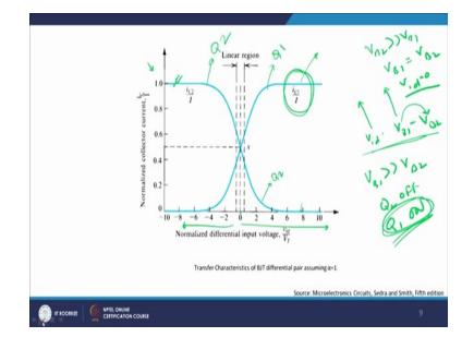
Now, with this knowledge which you have gained till now, right let me just therefore give you a small idea about the transfer characteristics. Now, on the y axis you will see it is basically the normalized collector current which means that collector current normalized with respect to the total current which is available to us and therefore the maximum I Can go is 1 and on the x axis we have V <sub>id</sub> by  $V_T$ ,  $V_{id}$  is basically the difference voltage of the base
