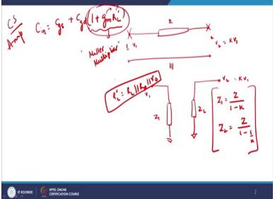
So, let us suppose I have I want to just refurbish the whole thing. So, I will let us have a two port network, this is port one and this is port two and I have V1 is the voltage source at port 1 and I say at port 2 the voltage V2 is equals to k \* V1, which means that the voltage at V2 is a function of V1, right. So, there is sort of feedback loop between nodes 2 and 1, right.
