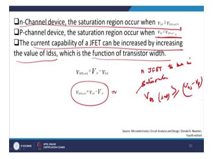
As I discussed with you in n channel JFET, therefore the saturation region occurs when  $V_{DS}$  is greater  $V_{DS}$  sat, exactly the same principle for a MOSFET, so I am going bit fast in this case because we are already deal with MOSFET in a detailed manner, conceptually, mathematically same as MOS device but cross section wise slightly difference in each operation value.
