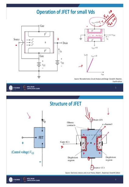
On the such a criteria, we will see (how those) how it works out or how it works in a general sense. So, before we move, so this is a structure which you see, as I discussed with you, the doping concentration here is pretty large, this is also doping concentration is pretty large and drain and source you have metal contact here. Now, as I discussed with you even a without application of any external source or external bias there will be obviously a depletion region is will be here, right.
