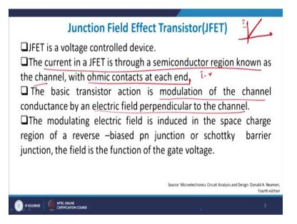
So, it is what we will doing here? So, again as have, as a MOS device, this also voltage control device which means that this basically again a voltage control current source. So, you will be applying a voltage and the current will be changing on the output side. So, the current in the JFET is therefore through a (resi) semi-conductor region known as channel and the with the ohmic contacts at each end, ohmic contacts means? Which follow I V current versus Voltage linear graph.
