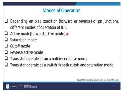
Now, therefore the various modes of operation are given as these are the various modes of operation right, depending upon the bias condition very simple straight forward. So there are two biases right, so I can have  $2^2$ , so I can have four sort of modes right.
