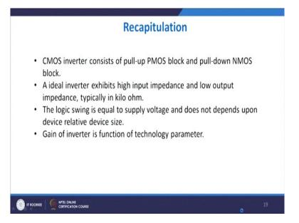
So let me recapitulate what we did. CMOS consists of PMOS block and NMOS block, an ideal inverter has got a high impedance and 0 output impedance. The logic swing is equal to supply voltage, it does not depend upon the device relative size and the gain the inverter is mostly a function of the technology.
