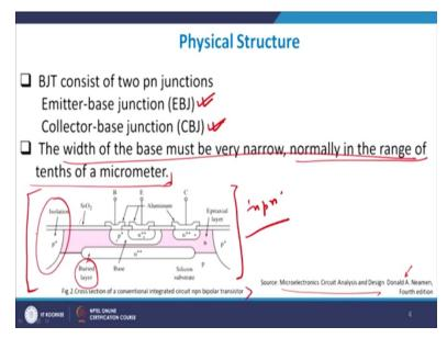
As I discussed with you therefore that the width of the base should be very narrow, right normally in the range of tenths of a micrometre and that is quite important and therefore the width of the base, right determines to what extent you will get the output current right. Just to give you a brief inside into this as we move along, but primarily the width of the base is a deciding factor as far as the total output current is available to you.
