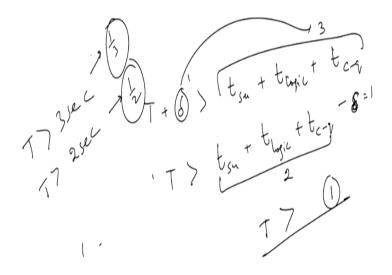
So this is the new value with you see now you see if this is true that t + delta should be greater than t setup + t logic +tcq then t should new inequality you should be t setup + t logic right +t2q – delta because this delta transfers to this side you get - delta right which means that in fact if you look very carefully a positive skew age your sequential logic because if it is – delta it basically means let us suppose this was 2 second now this will be just 1 second.
