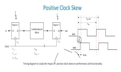
The rising clock edge is delayed by a positive  $\boldsymbol{\delta}$  at the second register.
