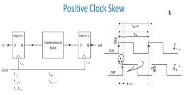
Timing diagram to study the impact of positive clock skew on performance and functionality.
