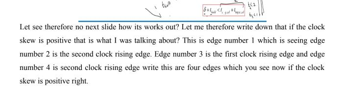
Then the time available for the signal to propagate from R1 to R2 is increased by the skew equals to delta I am clear like you get the point that since you are increasing the value of delta so the time available for you to propagate from this edge various sampling the data till this edge, till this edge so basically t clock + delta is total time available with you so if you remember the previous discussion.
