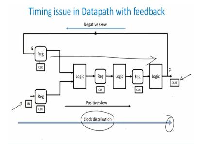
It is always advisable that when you do a feedback you try to do a negative skew because the data is moving in this direction, right and when you move the data is moving in this direction, right. If the clock which is movement in this the data and the clock are moving in the same direction primarily meaning that all your feedback forward arrangements in the forward direction will give you positive skew whereas all your feedbacks will give you a negative skew, fine.
