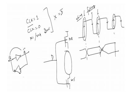
Which means that if you have a clock and the clock is this like this which is giving me a fixed value, then if it is a positive edge triggered clock then during the rising edge of the clock which is this or this you are able to sample the data. So the data was getting sample exactly at the rising edge of the clock, right. And the sampling was there provided you do not valid the set of time and whole time evaluations.
