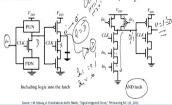
For example, you do have a this is suppose your latch, right. So this is one of your latch which is basically a negative latch and then you put input here and then depending upon the value of PUN suppose clock is equals to is high which means that this will be shorted. And therefore this will act as an inverter and in value will have an in minus or whatever by depending upon the value of the upon the logic gate a some value will be a stored here, right.
