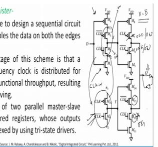
Let us suppose your clock is basically a high then M2 will be on and clock bar is low which primarily means M3 will be on. And therefore this set will be transparent and a mod X will be therefore equals to D bar which will be stored here. But if you see, if your clock is this is so what is happening in the first case is let me give an idea but if clock = 0, right. Let me again come back if clock equals to 1, then clock bar will be equals to 0.
