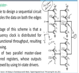
So what I am trying to tell you therefore is that if your design is such that you do have a clock here and a clock inverted register here, then I will be able to store the data at point Q in a much easier fashion and I can also make it transparent. So when the next clock cycle whatever the value of X is stored here will be transported to Q, right and that is the reason we get this type of what is known as at so this thing.
