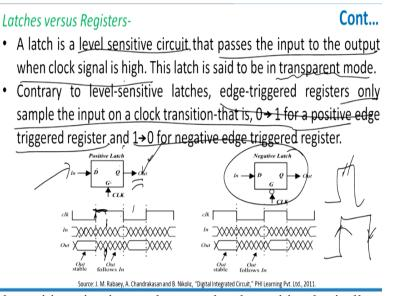
A latch is the level sensitive circuit so whenever level sensitive basically means this is level sensitive then edge means this is edge right so level sensitive circuit but passes the input to the output when the clock signal it is very straight forward. So when the clock is high it passes input to the ground input and output right and then in that state the latches said to be transparent mode right is known as transparent mode.
