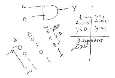
For example I have an AND gate right A and B are there so what is the truth table all of your aware of that why will be so A, B, C so if I draw the truth table i get right so this is the truth table as you get for the NAND gate which means that once your input pattern is fixed at A = B = 0 output as to be 0. Similarly if any on the 2 conditions 3 conditions are met output will be always equals to 0.
