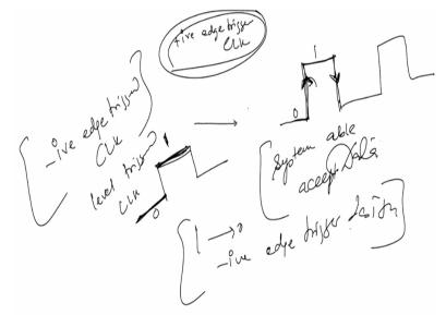
Suppose I have date coming right I defined a clock basically positive edge triggered design right let us suppose I define is known as the positive edge it basically means that when the clock is rising the positive edge which is this one right this is the falling edge again rising again falling so clock is going on during the rising edge of the clock the system is able to except data when the clock is rising.
